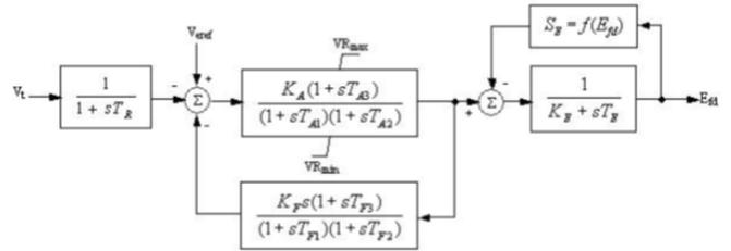
Figure 2: IEEE Type-AC5A excitation model
