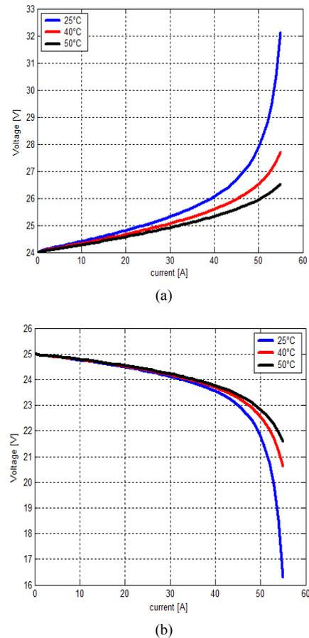
Figure 8: Variation of the voltage versus the current for different values of temperature: a) discharge mode; b) charging mode
