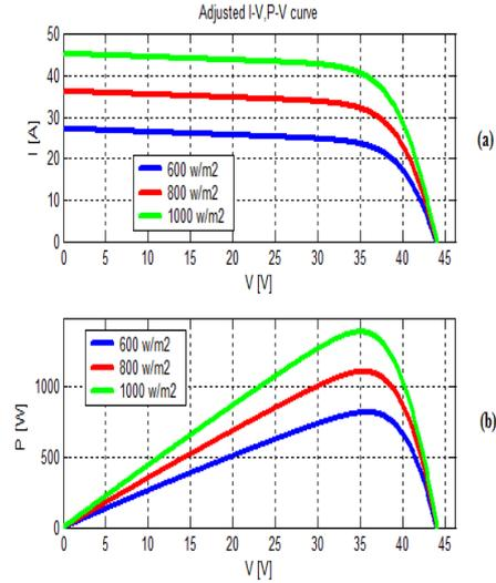
Figure 4: I–V and P–V curves of a PV generator at variable irradiation and constant temperature
