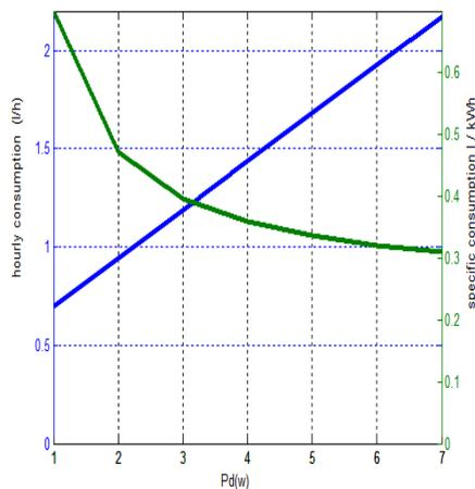
Figure 10: Consumption of the diesel generator as a function of the power produced
