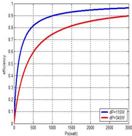
Figure 9: The efficiency of the inverter as function of the power demand
