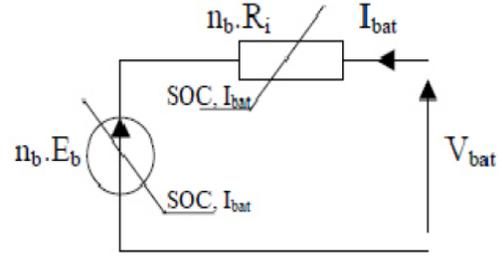
Figure 3: Equivalent electrical diagram of  $n_b$  battery elements in series
