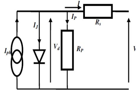
Figure 2: The Equivalent electrical circuit of a photovoltaic cell
