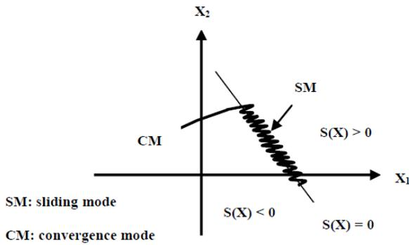
Figure 9: Trajectory mode in the phase plane
