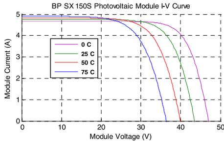
Figure 4: I-V curves of BP SX 150S PV module at various sun radiations simulated with the MATLAB model
