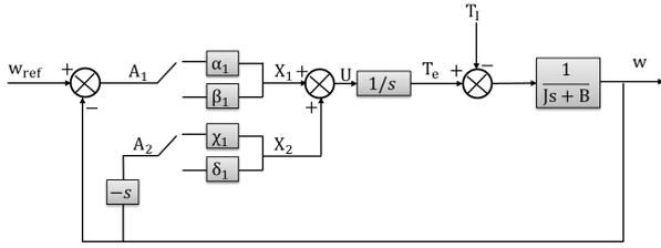
Figure 10: Simplified model of the drive system
