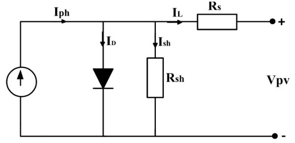
Figure 2: Equivalent circuit of PV array
