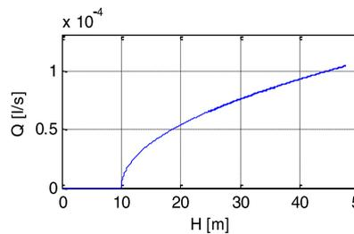
(d) Variation in the head and flow of PV pumping system
