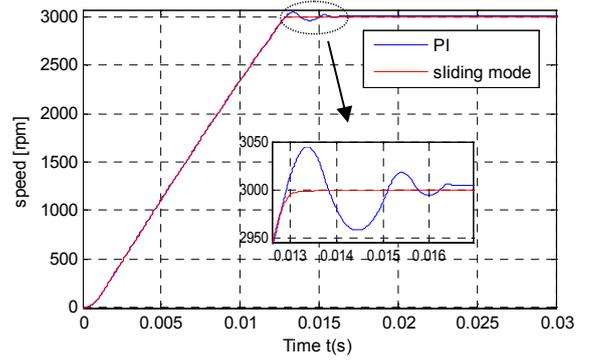
Figure 11: Comparative response of the speed control using sliding mode and PI controllers
