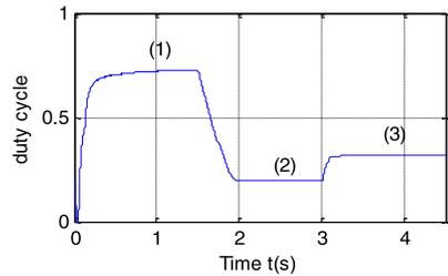
(b) Duty cycle response of PV pumping system
