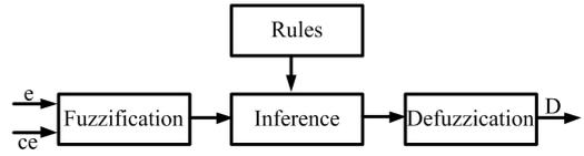
Figure 6: Diagram of fuzzy logic controller
