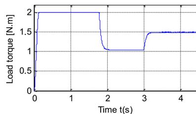
(e) Load torque of PV pumping system
