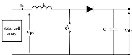
Figure 5: Basic circuit of the boost chopper
