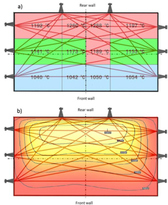
Figure 2: AGAM results presentation a) average temperature of sub-areas; b) isotherms plot
