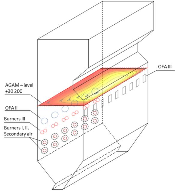
Figure 6: Fuel and air distribution system in K-4 boiler, in Rybnik Power Plant
