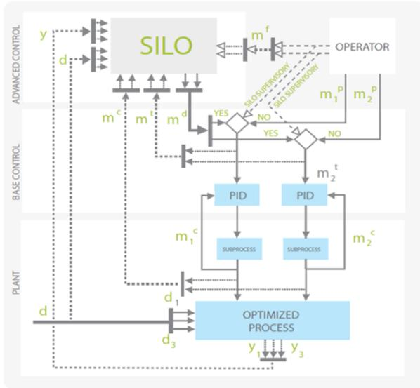
Figure 3: The architecture of SILO implementation in layered control structure
