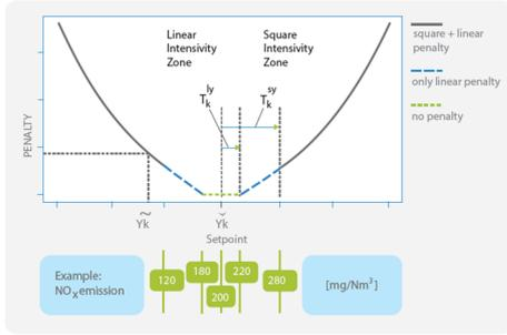
Figure 5: Example settings of penalty function for NO<sub>x</sub>
