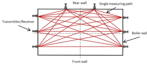
Figure 1: An example of industrial application of an AGAM system
