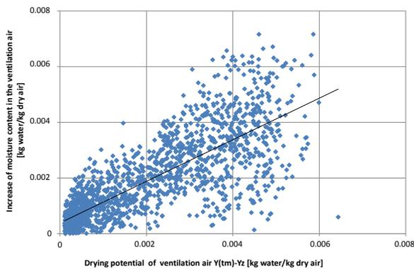
Figure 1: Increase in moisture content in the ventilation air as a function of drying potential for that air during the analyzed operating cycle of the test facility—experimental data
