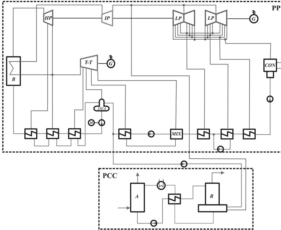
Figure 1: Object of the research – power plant coupled with a CO<sub>2</sub> separation unit
