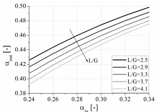
Figure 3:  $\alpha_{in}$  vs  $\alpha_{out}$  for selected values of  $L/G$  in the absorber column
