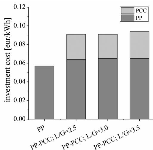
Figure 7: Investment cost of PP with and without PCC related to the 1 kW power
