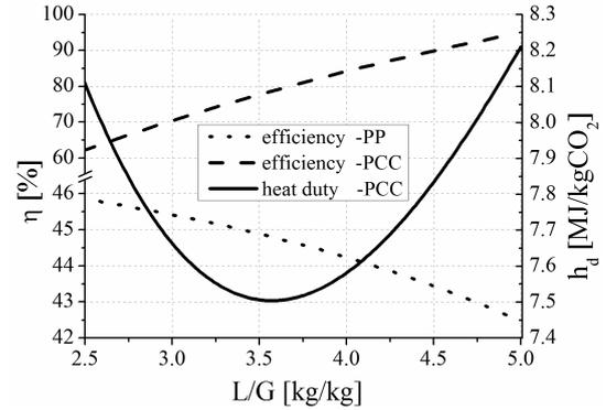
Figure 2: CO<sub>2</sub> capture and PP efficiencies and heat duty vs  $L/G$ .
