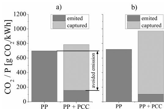
Figure 8: Comparison of amount of CO<sub>2</sub> produced in the installation with and without PCC, IMC results (a) and data taken from work [35] (b), both figures share the same scale
