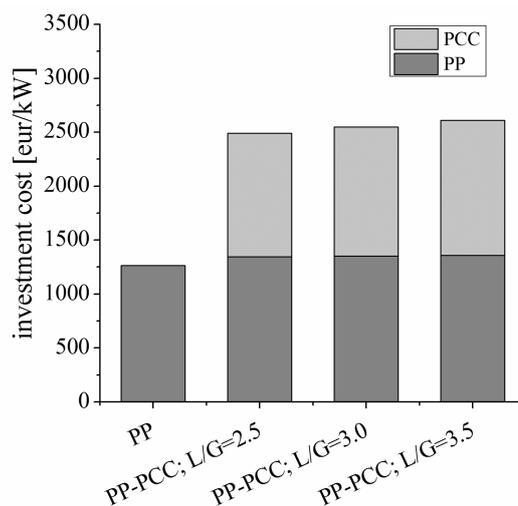
Figure 4: Investment cost of PP with and without PCC related to 1 kW power
