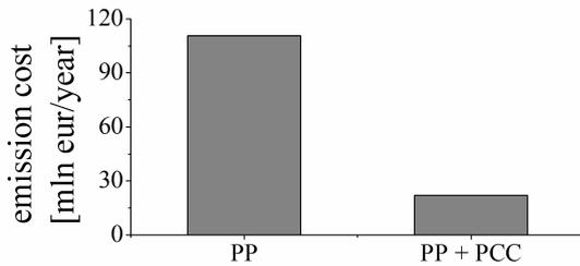
Figure 9: Comparison of CO<sub>2</sub> emission from PP without and with PCC in a one year period.
