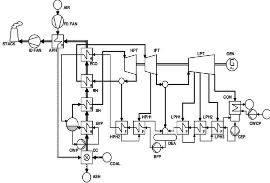
Fig.1. Schematic diagram of the existing steam power plant
