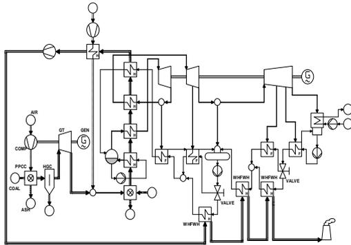
Fig.2. Schematic diagram of the repowered power plant
