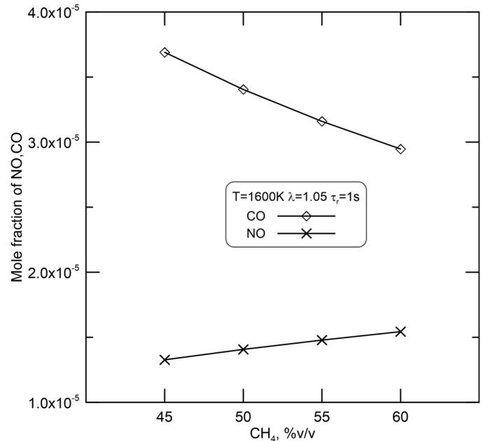
Figure 6: Influence of CH<sub>4</sub> content in the biogas on the mole fraction of CO and NO
