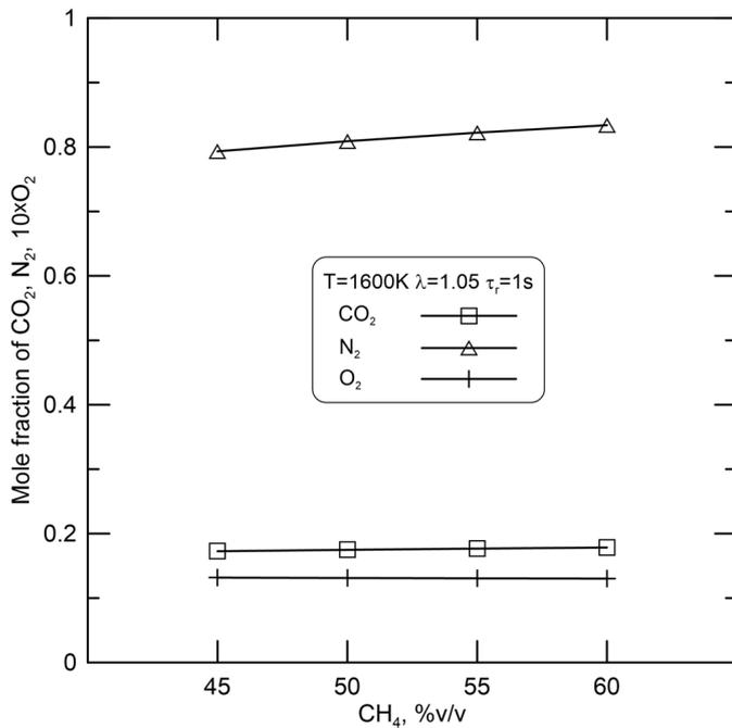
Figure 7: Influence of CH<sub>4</sub> content in the biogas on the mole fraction of CO<sub>2</sub>, N<sub>2</sub> and O<sub>2</sub>
