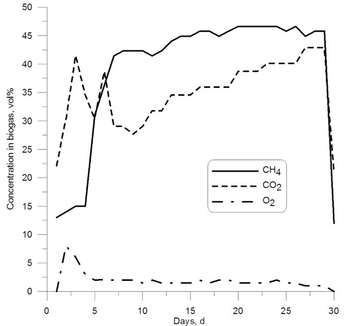
Figure 4: Concentrations of components in biogas
