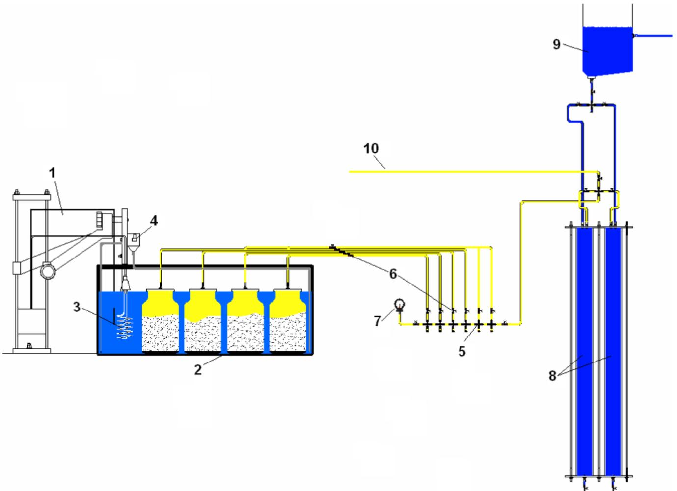
Figure 3: A schematic representation of the test stand with a 2 liter fermenter
