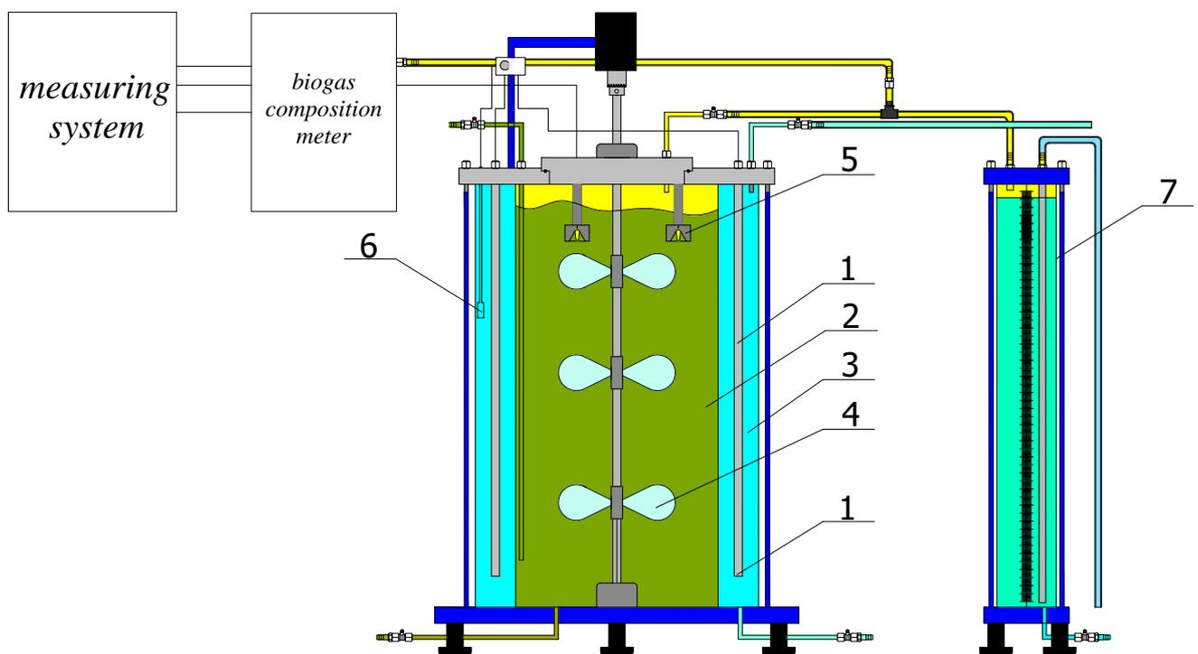
Figure 2: A schematic representation of the test stand with a 20 liter fermenter
