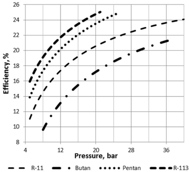
Figure 13: Power efficiency of the ORC system for selected low-boiling fluids (helium temperature before the compressor—110°C) ( $p_{de} = 80$  bar)—Variant II
