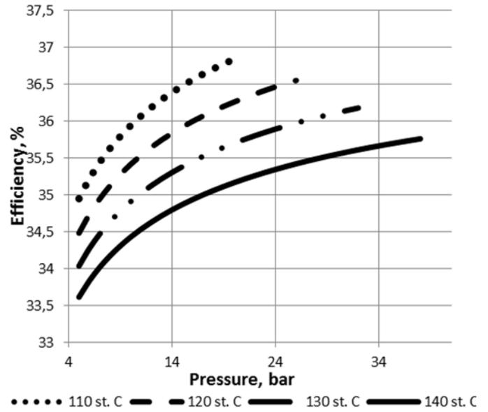
Figure 11: Power efficiency of the system for assumed values of the temperature of helium before the compressor (ethanol,  $p_{4e} = 80$  bar)—Variant II
