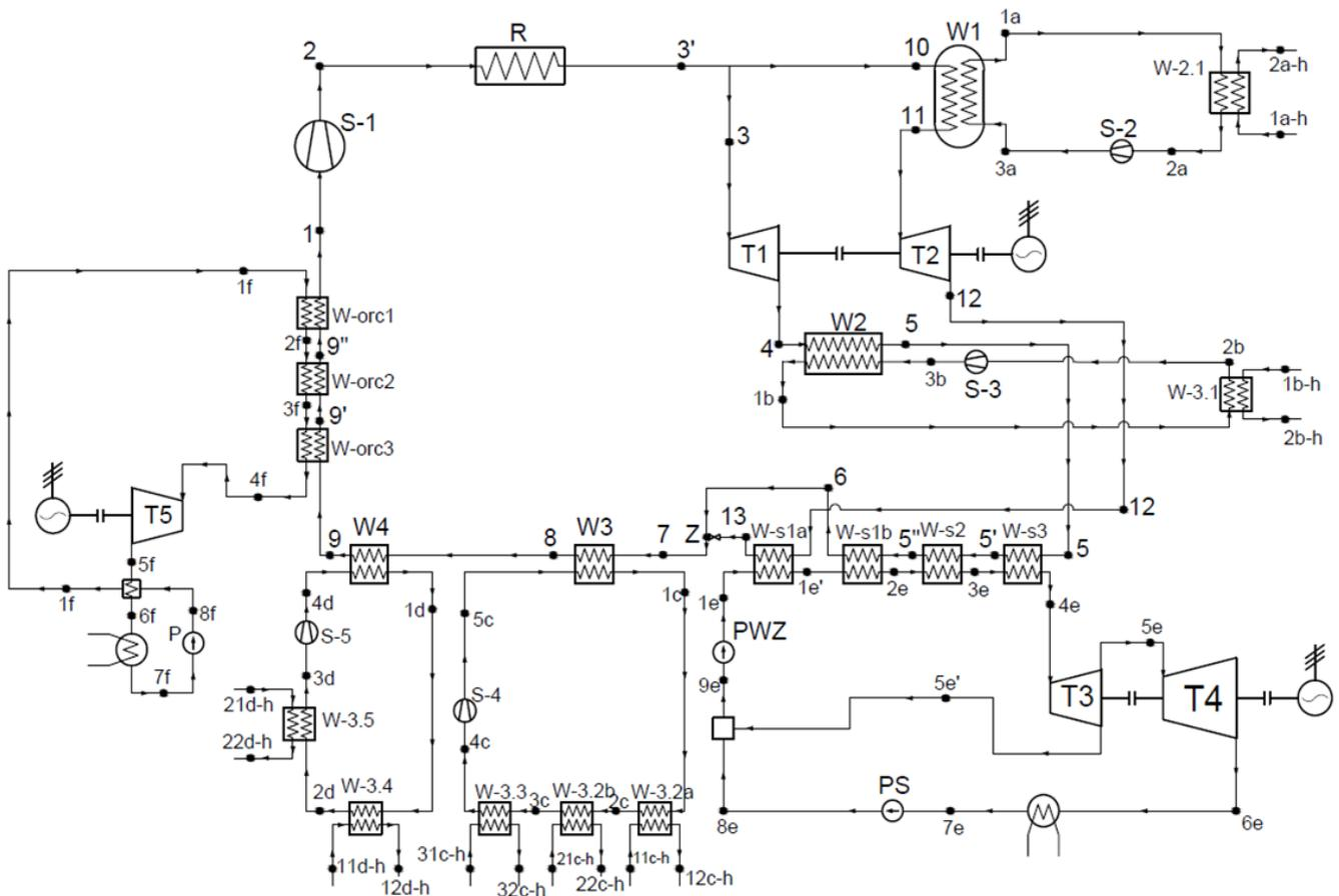
Figure 1: Diagram of the energy cogeneration system with the high-temperature nuclear reactor—Variant I
