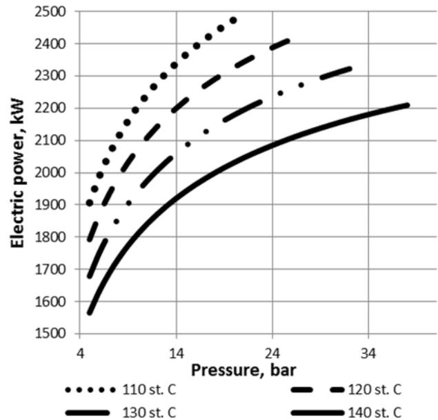
Figure 8: Net electric power generated in the ORC system for assumed values of the temperature of helium before the compressor (ethanol,  $p_{4e} = 80$  bar)—Variant II
