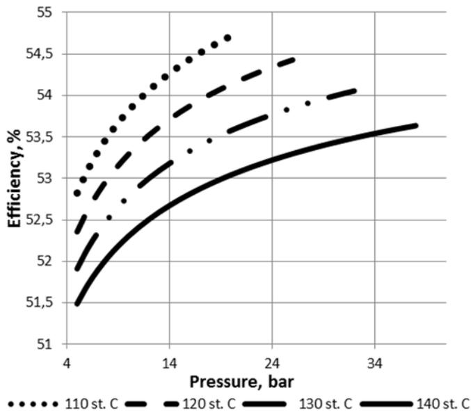
Figure 10: Efficiency of the cogeneration system for assumed values of the temperature of helium before the compressor (ethanol,  $p_{4e} = 80$  bar)—Variant II
