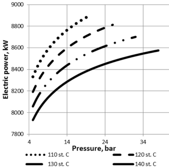
Figure 7: Total net electric power generated in the cogeneration system for assumed values of the temperature of helium before the compressor (ethanol,  $p_{4e} = 80$  bar)—Variant II
