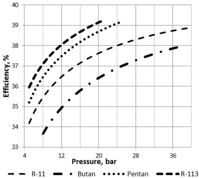
Figure 14: Total power efficiency of the system for selected low-boiling fluids (helium temperature before the compressor—110°C) ( $p_{de} = 80$  bar)—Variant II
