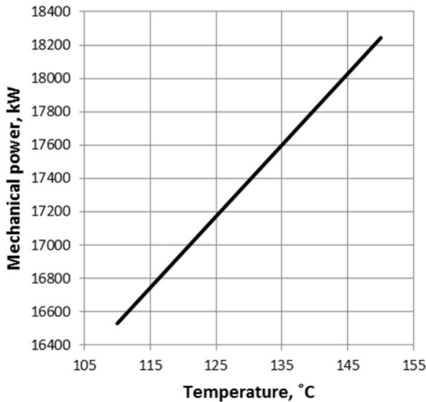
Figure 5: The compressor driving mechanical power depending on helium temperature at the device inlet—Variant II
