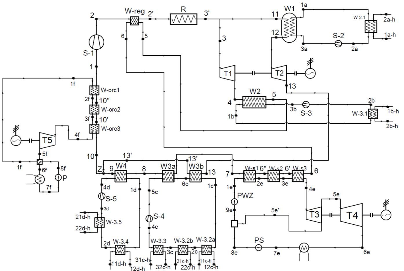
Figure 2: Diagram of the energy cogeneration system with the high-temperature nuclear reactor—Variant II
