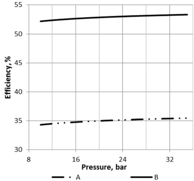
Figure 4: Efficiency of the cogeneration system (A) and the system total power efficiency (B) for assumed values of the low-boiling fluid vapor pressure (ethanol,  $p_{Ae} = 80$  bar,  $t_1 = 150^\circ\text{C}$ )—Variant I
