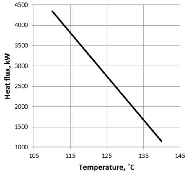
Figure 6: The regeneration heat flux depending on helium temperature at the inlet—Variant II
