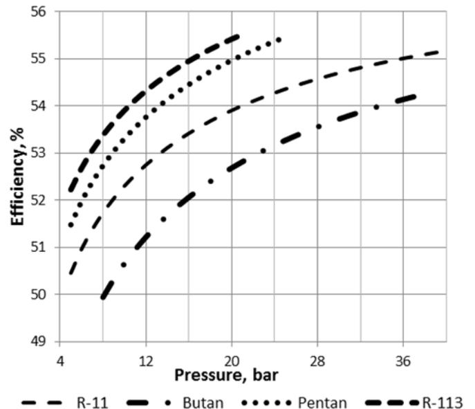
Figure 12: Power efficiency of the cogeneration system for selected low-boiling fluids (helium temperature before the compressor—110°C) ( $p_{4e} = 80$  bar)—Variant II
