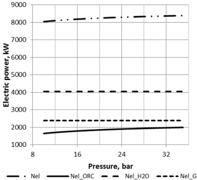
Figure 3: Total net electric power generated in the cogeneration system, electric power of the OCR system, electric power of the vapor cycle for assumed values of the low-boiling fluid vapor pressure (ethanol,  $p_{Ae} = 80$  bar,  $t_1 = 150^\circ\text{C}$ )—Variant I
