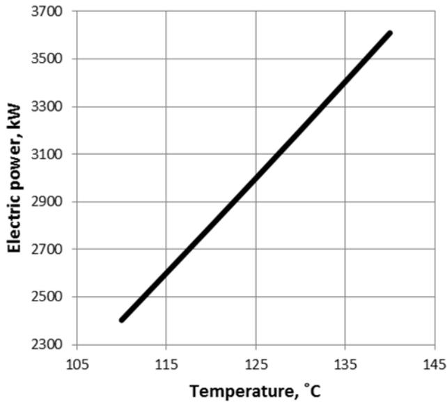
Figure 9: Net electric power generated in the water vapor system for assumed values of the temperature of helium before the compressor—Variant II
