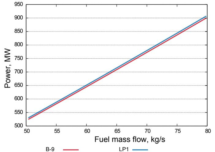
Figure 4: Changes in the power generated, depending on the fuel supply
