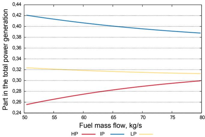
Figure 9: Ratios of each part of the steam turbine in total power generation
