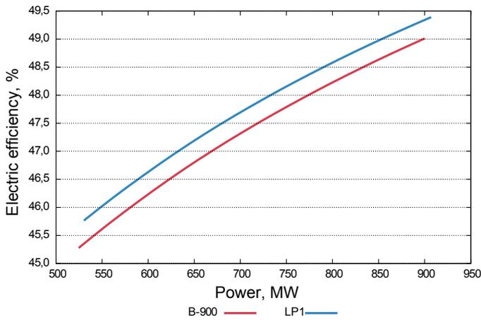
Figure 6: The efficiency of power generation depending on the power generated in both cases
