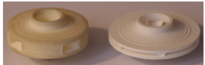
Figure 5: Two impellers with a different structure but similar pumping parameters
