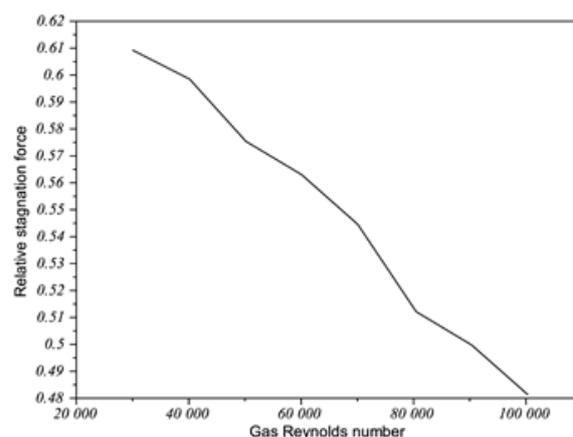
Figure 6: Ratio of stagnation force to surface tension force versus gas Reynolds number for air-water annular flow in 12.7 mm/31.75 mm annulus at atmospheric pressure; contact angle 24.5°C
