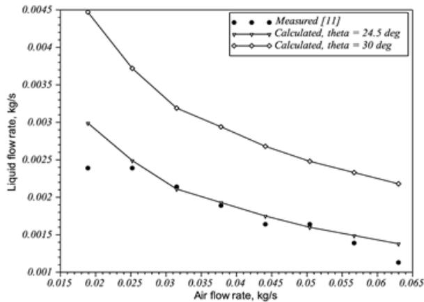
Figure 4: Minimum liquid film flow rate as a function of air flow rate. Comparison of predictions with experimental data [11]
