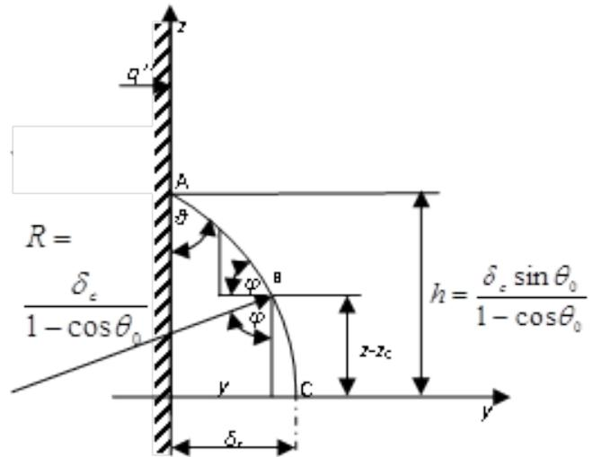
Figure 2: Assumed curvature of the leading edge of the liquid film
