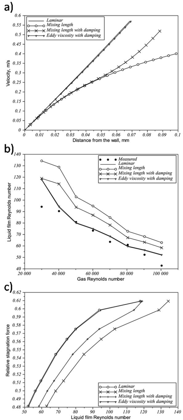
Figure 5: Influence of turbulence models on dry patch re-wetting in air-water annular flow in 12.7 mm/31.75 mm annulus at atmospheric pressure and contact angle 24.5°C: velocity profiles in liquid film (a), minimum re-wetting liquid film Reynolds number as a function of gas Reynolds number (b), ratio of stagnation force to surface tension force as a function of the liquid film Reynolds number (c)
