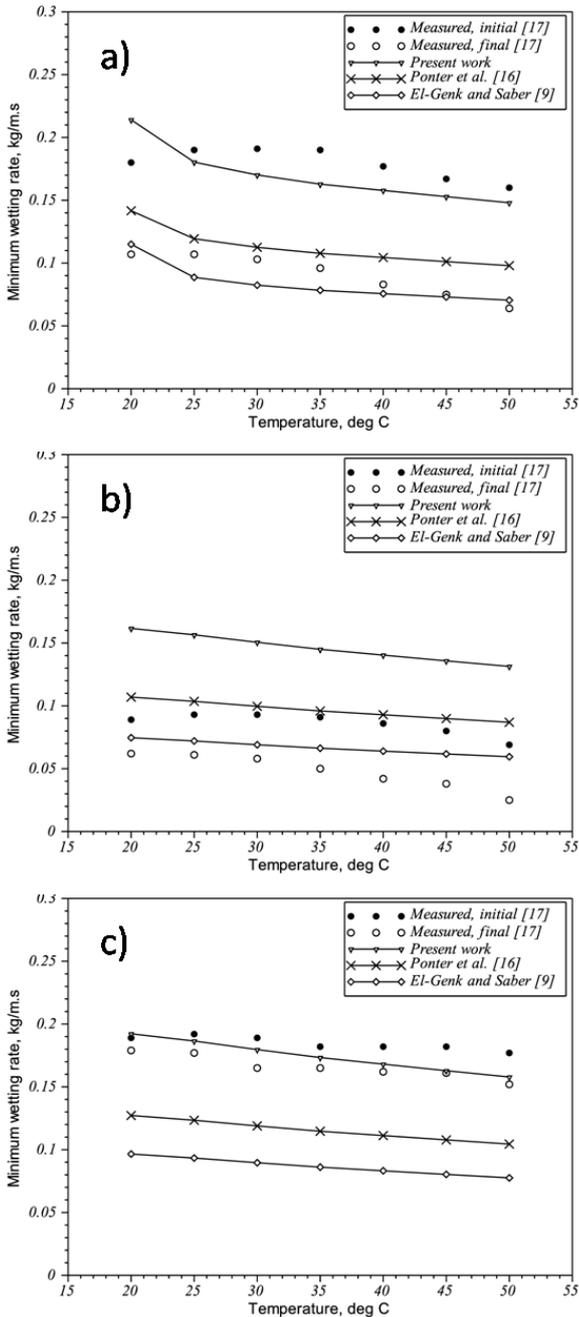
Figure 3: Prediction of the minimum wetting rate of liquid film flowing down a: copper surface (a), stainless steel surface (b), Perspex surface (c)
