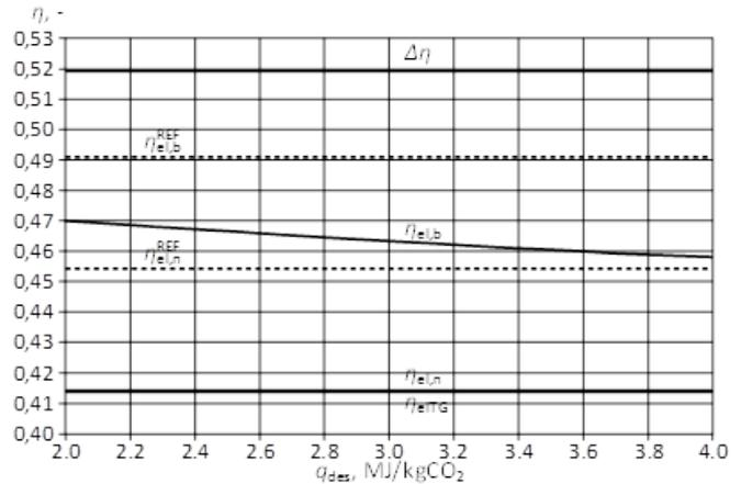
Figure 3: Efficiency characteristic as a function of heat demand for the desorption process
