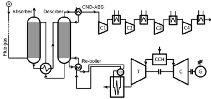
Figure 2: Diagram of CO<sub>2</sub> separation unit
