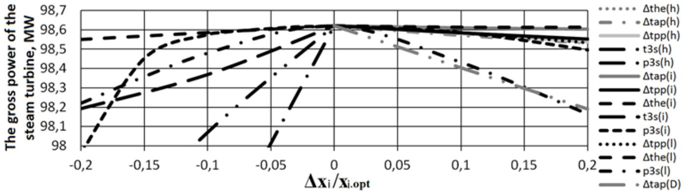
Figure 7: Sensitivity analysis for a triple-pressure combined cycle power plant with the steam reheat integrated with CCS
