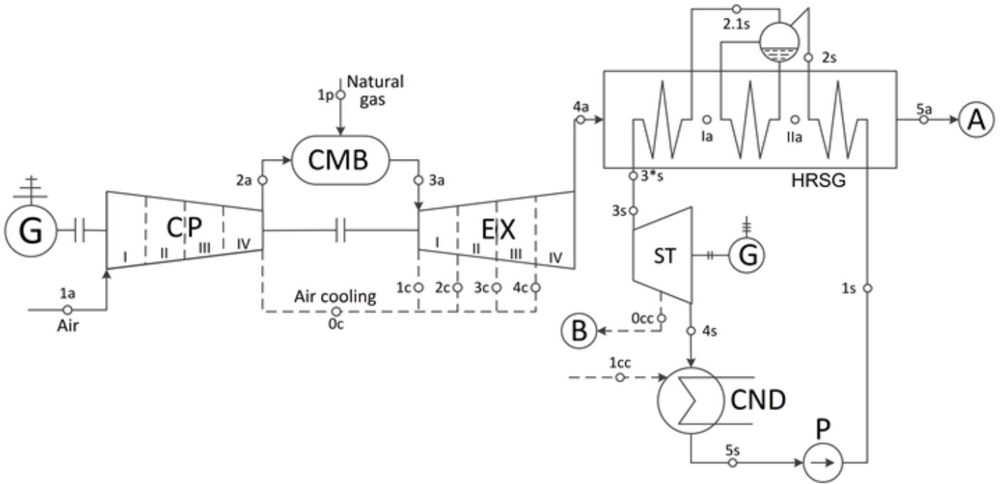
Figure 1: Schematic diagram of a single-pressure combined cycle power plant (1P)(G—generator, CND—condenser, P—condensate pump, SP—steam turbine, HRSG—heat recovery steam generator, A—flue gas stream, B—steam stream)
