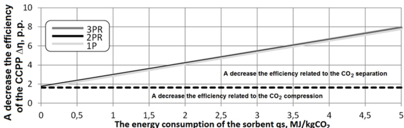
Figure 9: The decrease in efficiency of the units as a function of sorbent energy consumption
