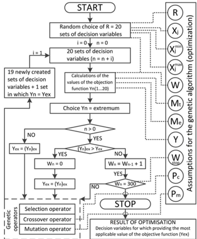
Figure 5: Block diagram of the genetic algorithm
