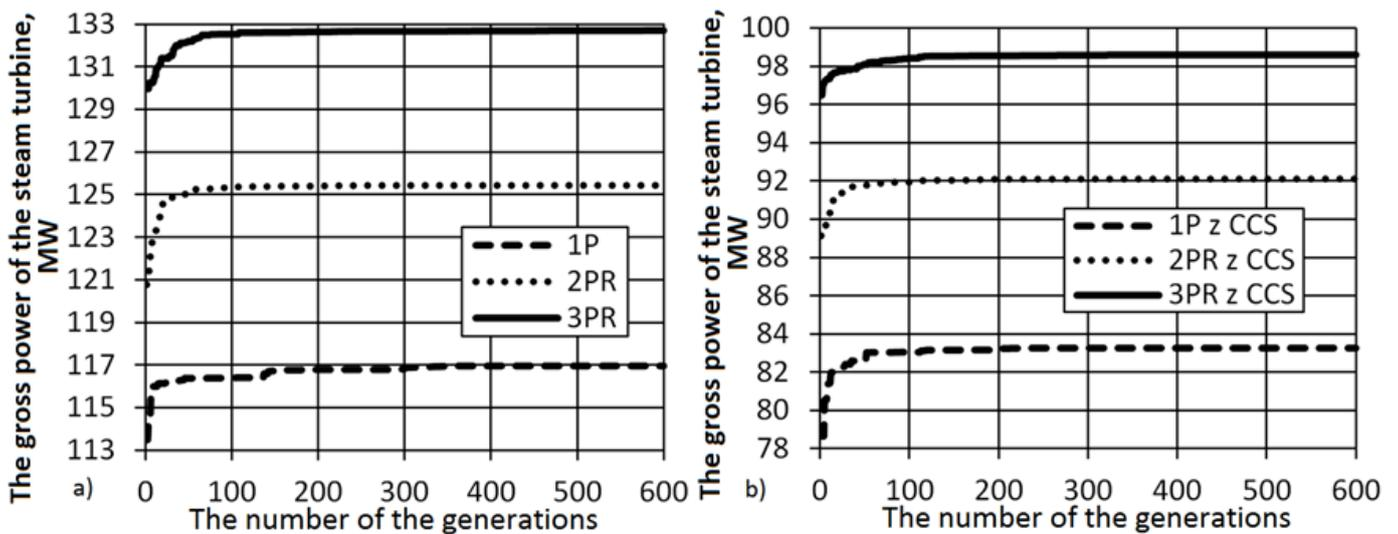
Figure 6: Extreme objective function values generated by the genetic algorithm for: a) CCPP without CCS, b) CCPP with CCP
