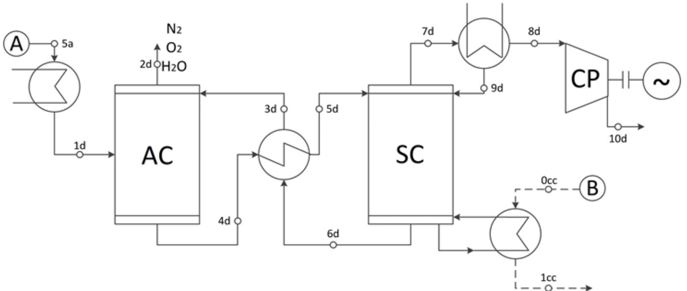
Figure 4: The system of CO<sub>2</sub> separation and preparation for transport (AC—absorber column, SC—stripper column, CP—CO<sub>2</sub> compressor, A—flue gas from the HRSG, B—steam flow from steam turbine bleed)
