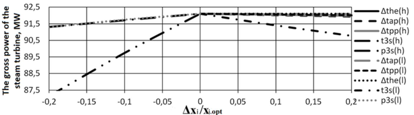
Figure 8: Sensitivity analysis for a double-pressure combined cycle power plant with the steam reheat integrated with CCS
