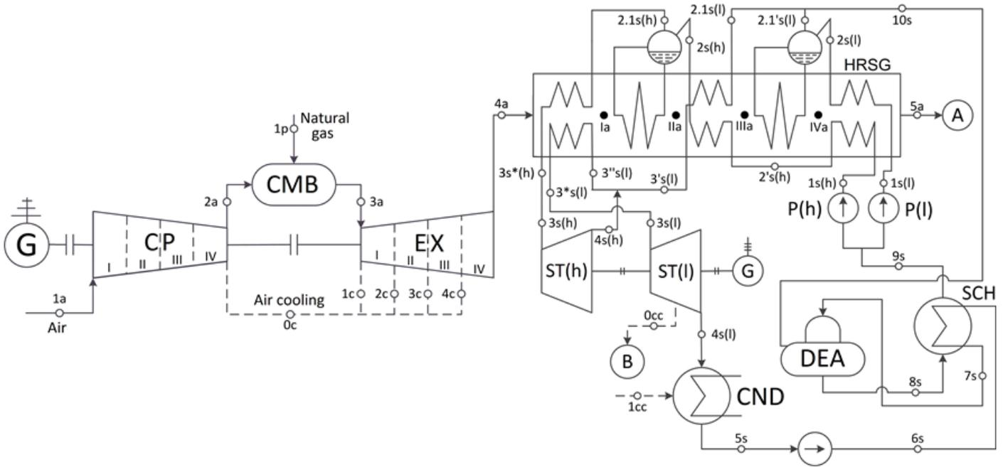
Figure 2: Schematic diagram of a double-pressure combined cycle power plant with a steam reheater (2PR)
