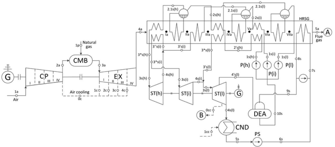
Figure 3: Schematic diagram of a triple-pressure combined cycle power plant with a steam reheater (3PR)
