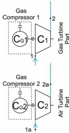
Figure 2: Gas-air system driving working machinery—a variant with two compressors
