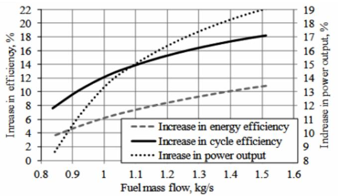
Figure 14: Increment in gas-air system efficiency and mechanical power output compared to a simple gas turbine unit for various values of fuel mass flow
