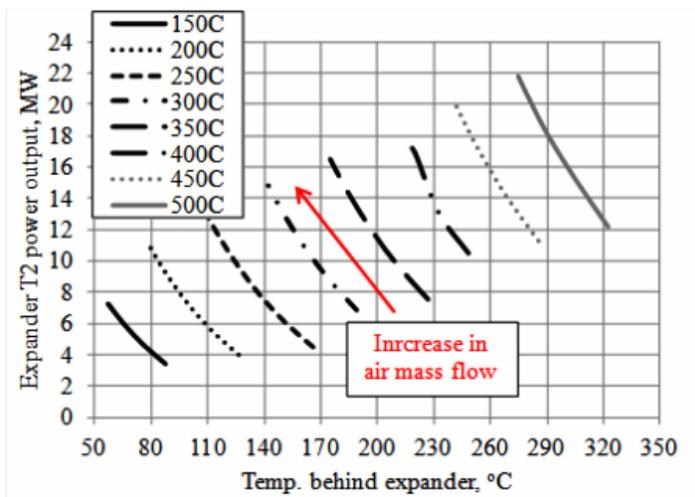
Figure 12: The dependence of the power output of the gas-air system air-part expander on temperature values after the air expander
