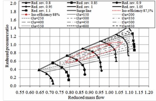
Figure 5: The compressor example characteristic with temperature values (in °C) before the expander
