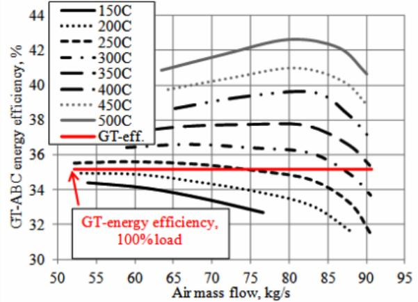
Figure 7: Gas-air system efficiency depending on the air mass flow
