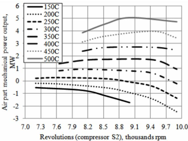
Figure 10: Power generated by the air part depending on the air turbine system rotational speed
