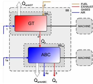
Figure 4: Gas-air system block diagram with balance boundaries
