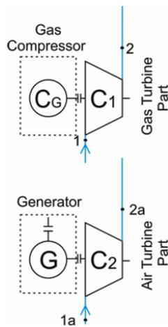
Figure 3: Gas-air system driving working machinery—a variant with a compressor and generator
