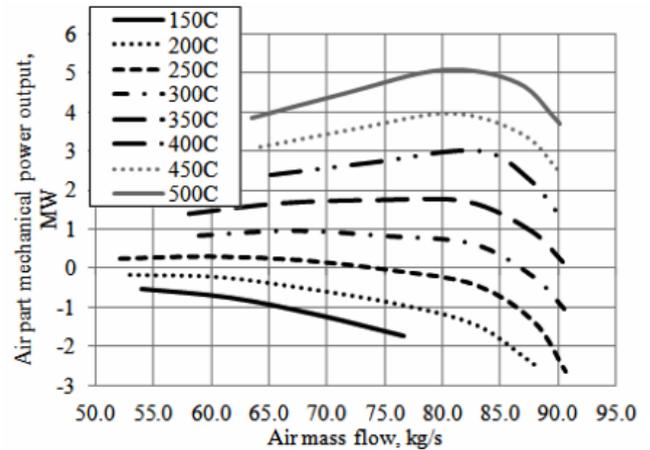
Figure 8: Gas-air system power output depending on the air mass flow
