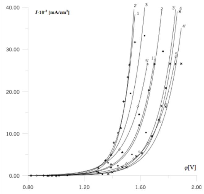
Figure 1: Polarization curves of electrooxidation of detergent SYNTANOL DS-10 (1'-5') and 0.01% emulsion of crude oil (1-5) in various concentration of electrolyte (H<sub>2</sub>SO<sub>4</sub>): 1,1'—0.01N; 2,2'—0.05N; 3,3'—0.1N; 4,4'—1.0N; 5,5'—5.0N
