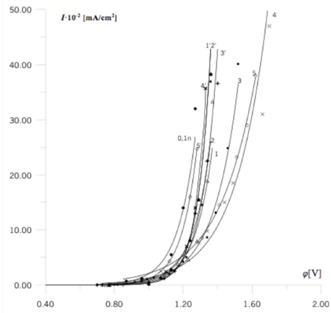
Figure 2: Polarization curves of electrooxidation of detergent SYNTANOL DS-10 (1'-5') and an emulsion of crude oil (1-5) in 0.1n concentration of electrolyte  $\text{H}_2\text{SO}_4$  (at 65°C): 1.1'—0.0025%; 2.2'—0.005%; 3.3'—0.010%; 4.4'—0.025%; 5.5'—0.050%
