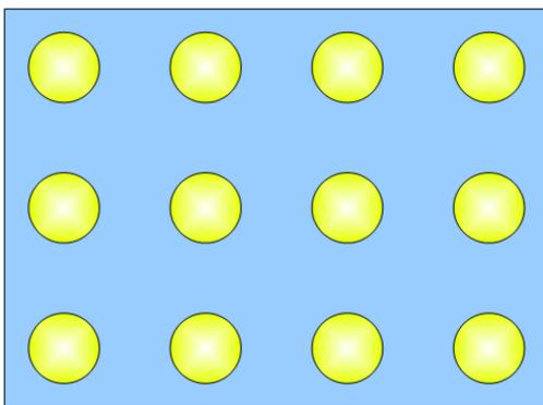
Figure 2: Spherical particles arranged in simple cubic array embedded in a continuous matrix, as considered by Rayleigh.
