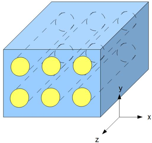
Figure 3: The schematic of the second type composite medium considered by Rayleigh, consisting of parallel cylinders embedded in a continuous matrix.
