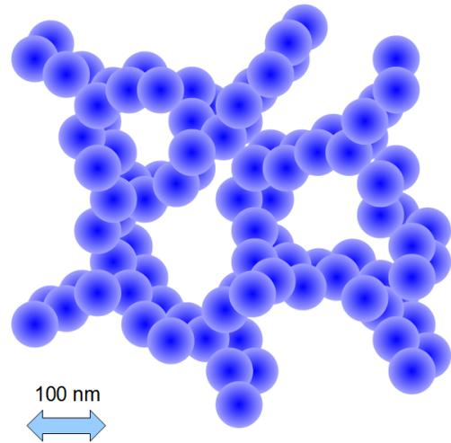
Figure 9: The schematic of an aerogel nanostructure. Silica aerogels obtained by sol-gel process and supercritical drying techniques are nanoporous, low-density, non-crystalline materials with large specific surface areas [35].
