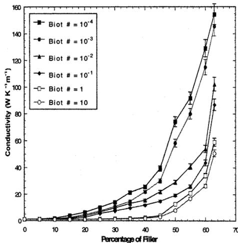
Figure 7: The effective thermal conductivity of alumina filler particles in the polyethylene matrix as a function of filler volume fraction for different Biot numbers<sup>1</sup> [4].
