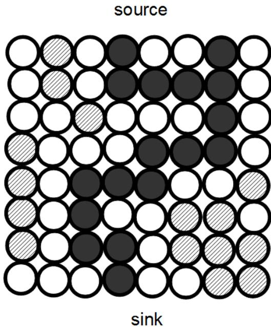
Figure 5: A scheme of heat transfer enhancement, in particulate composite material, due to percolation. High-conductivity particles, forming a continuous conductive chain from source to sink, are depicted as black. White is for low-conductivity particles, and hatching is for high-conductivity particles which do not form a continuous chain from source to sink.
