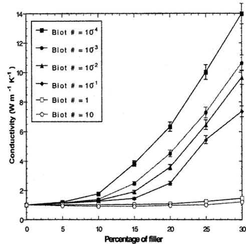
Figure 8: The effective thermal conductivity of alumina filler particles in the polyethylene matrix as a function of filler volume fraction for different Biot numbers. Blow-up for low volume fractions<sup>2</sup> [4].
