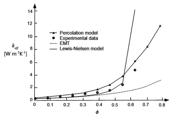
Figure 6: Effective thermal conductivity of bimodal distribution of  $\text{Al}_2\text{O}_3$  filler (65:9  $\mu\text{m}$ ) in a polyethylene matrix as predicted by different models, compared with experimental results.  $\phi$  – filler volume fraction Adopted from [10].
