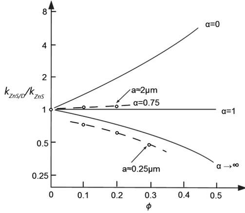
Figure 4: The ratio of ZnS/diamond composite thermal conductivity to the conductivity of pure ZnS matrix as a function of diamond filler volume fraction  $\phi$ , where: dashed line – measurement results for two sizes of filler particles, solid line – theoretical predictions based on (10),  $a$  – average particle radius. Adopted from [3].
