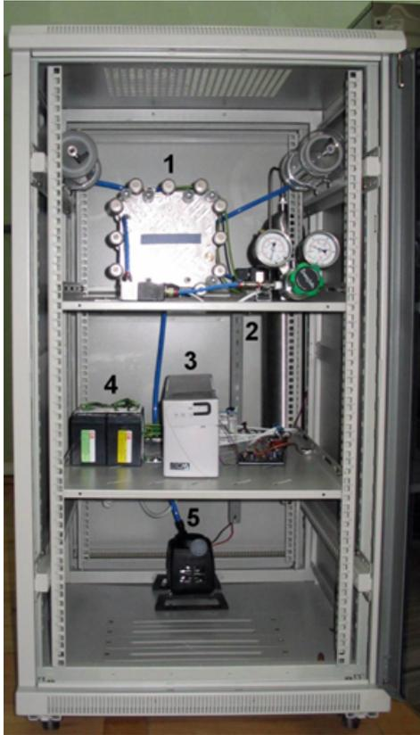
Figure 1: UPS with fuel cell module, 1—fuel cell stack, 2—hydrogen container and gas pressure reducer, 3—power controller with DC/AC converter, 4—batteries, 5—air compressor
