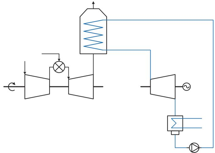
Figure 1: Simplified layout of offshore combined cycle with once-through HRSG
