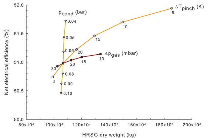
Figure 4: Sensitivity of flue gas pressure drop, pinch-point temperature difference, and condensing pressure on HRSG dry weight and net electrical efficiency
