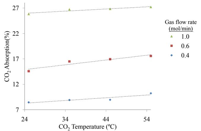
Figure 5: Heating effect on carbon dioxide absorption ( $L = 1.4$  liters/min)
