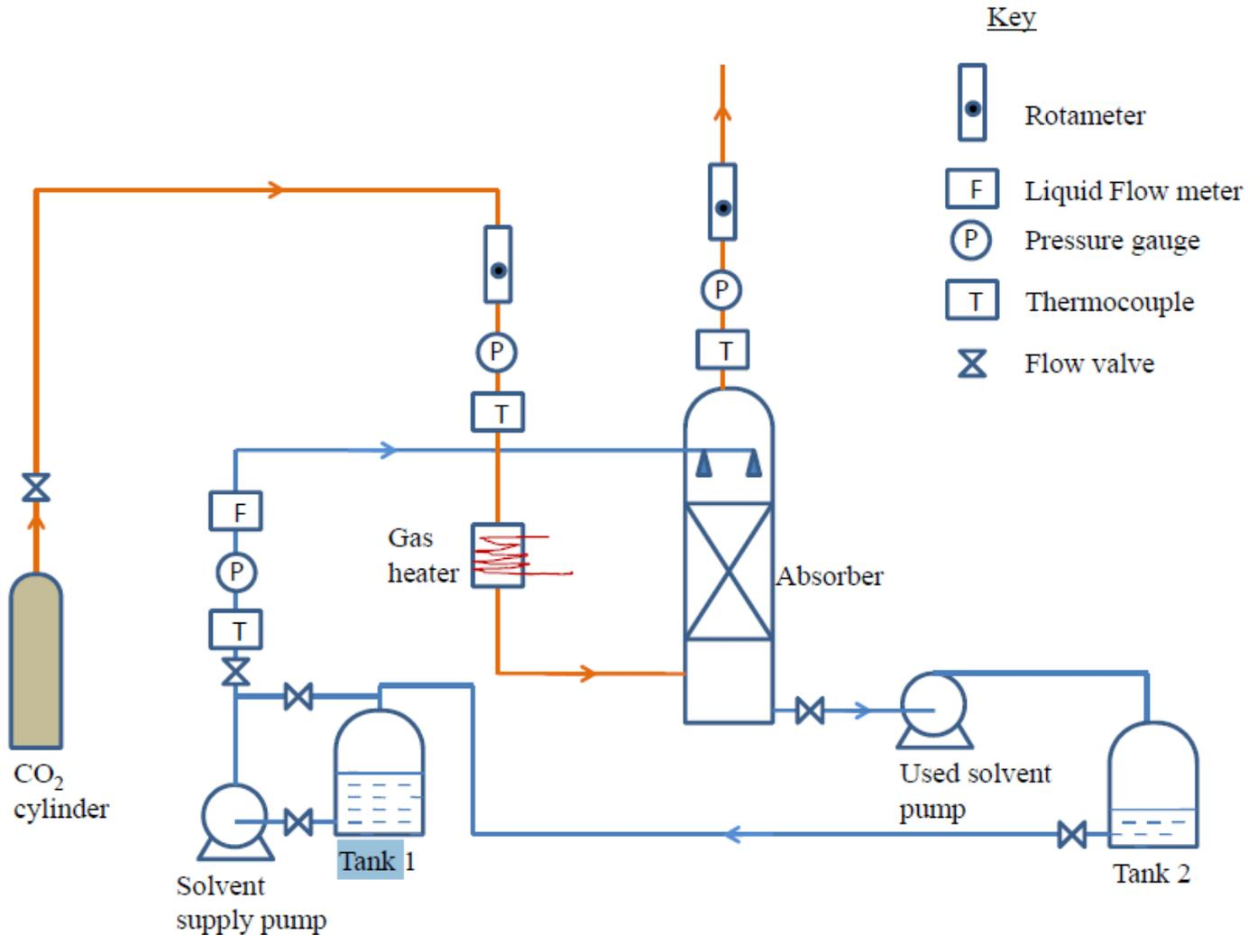
Figure 1: Layout of the CO<sub>2</sub> absorption plant
