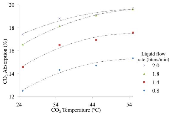
Figure 4: Heating effect on carbon dioxide absorption ( $G = 0.6$  mol/min)
