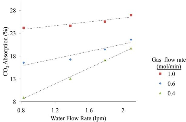
Figure 2: Absorption profiles due to liquid loading
