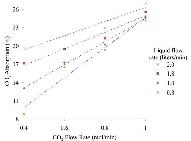
Figure 3: Absorption profiles due to gas loading
