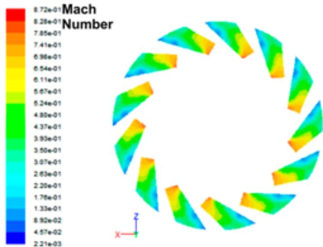
Figure 7: Contours of Mach Number in the diffuser
