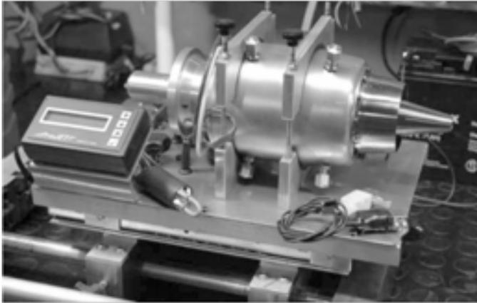
Figure 1: Photo of the GTM-120 turbo-jet engine
