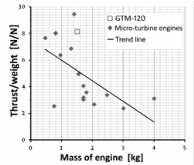
Figure 12: Thrust-weight ratio versus mass of engine
