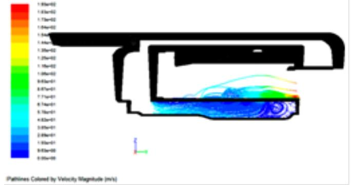
Figure 19: Pathlines of velocity magnitude showing the air flow through the annulus and through the second row of holes into the liner
