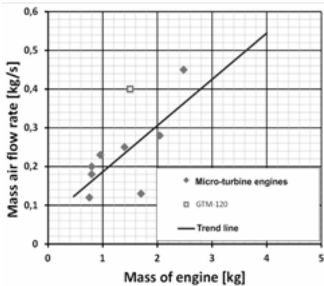
Figure 11: Air mass flow versus mass of different micro-turbine engines
