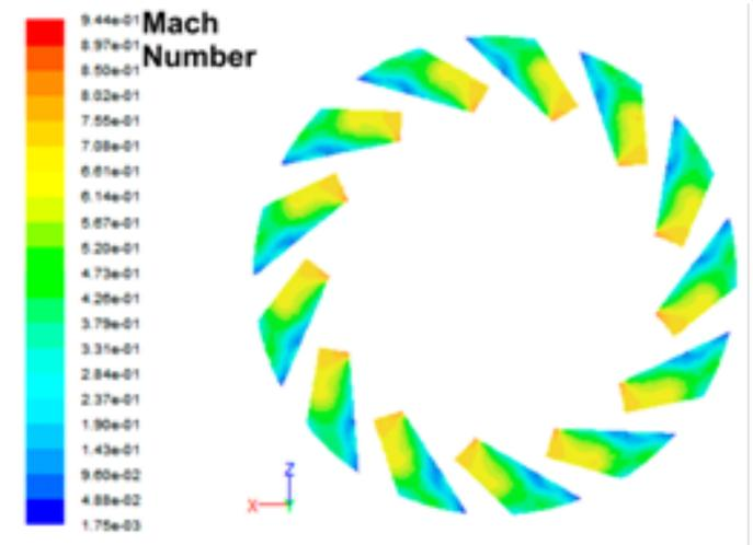
Figure 9: Contours of Mach Number in the diffuser
