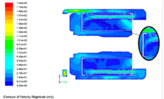
Figure 14: Contours of velocity magnitude in the combustor
