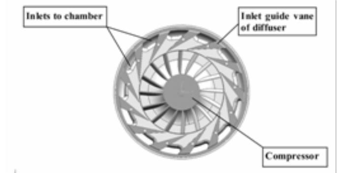
Figure 3: Cross-section of the GTM-120 turbo-jet engine showing the position of the compressor diffuser vanes
