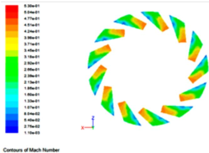
Figure 13: Contours of Mach number in the diffuser
