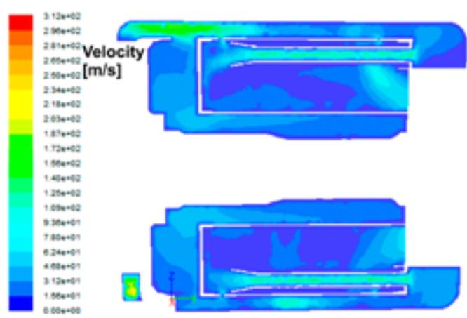
Figure 8: Contours of velocity magnitude in the combustor
