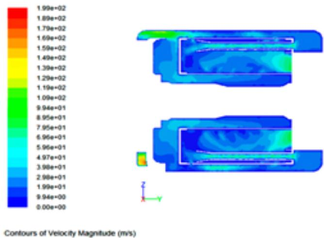
Figure 18: Contours of velocity magnitude in the combustor
