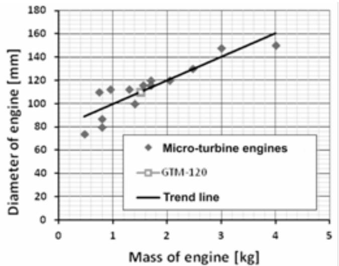
Figure 4: Diameter of engine versus mass of engine
