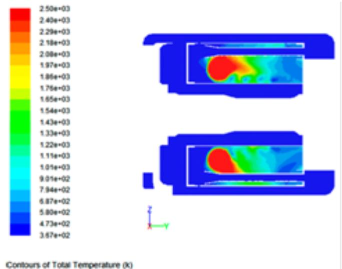
Figure 16: Contours of temperature in the combustor
