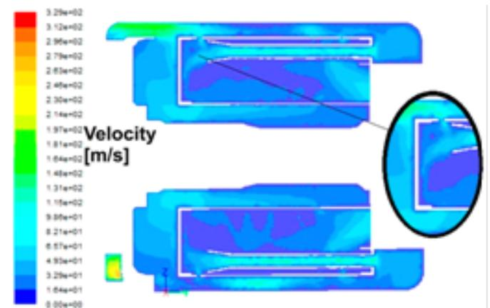
Figure 10: Contours of velocity magnitude inside combustor
