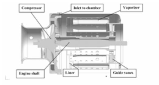
Figure 2: Cross-section along the length of the GTM-120 turbo-jet engine
