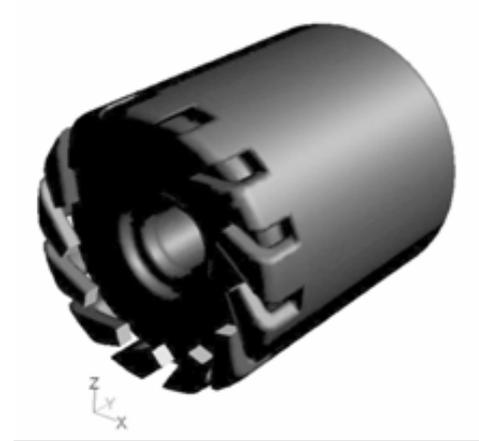
Figure 5: Geometry of the combustion chamber prepared for numerical simulations
