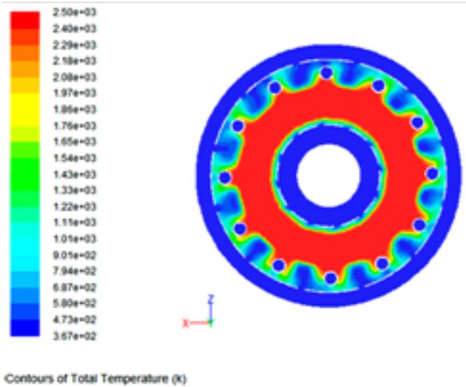
Figure 17: Contours of temperature in cross sections of the combustor
