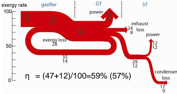
Figure 4: Theoretical energy/exergy flow of the Advanced IGCC system with exergy recuperation [6]. The net efficiency in brackets takes oxygen generation power into consideration.
