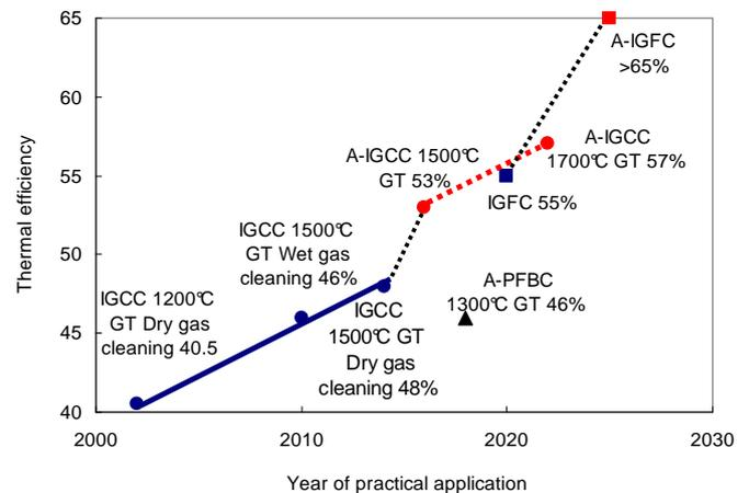
Figure 1: Performance projection of future coal based power plants [6]
