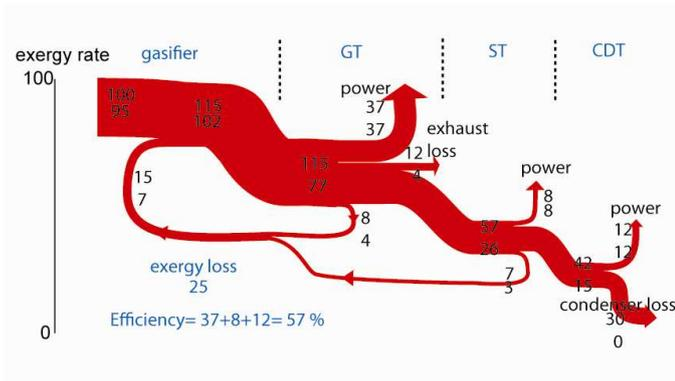
Figure 10: Energy/Exergy flow of the A-IGCC model
