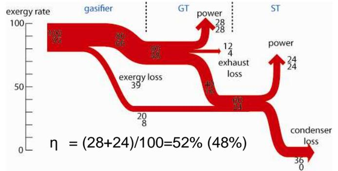
Figure 3: Theoretical energy/exergy flow of a conventional cascading IGCC system [6]. The net efficiency in brackets takes oxygen generation power into consideration.
