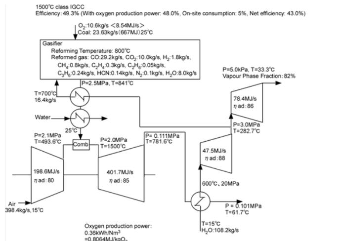
Figure 7: Performance and process flow diagram of IGCC model
