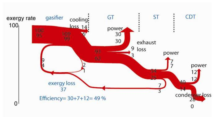
Figure 9: Energy/Exergy flow of the IGCC model
