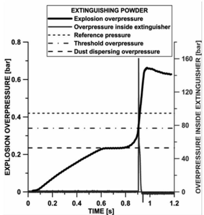
Figure 12: Courses of the overpressure inside the 1.3 m<sup>3</sup> test chamber during explosion of corn starch dust ( $C = 0.2 \text{ kg/m}^3$ ) and inside the extinguisher. Activation from photodiode signal at the level of 1.0 V. Explosion overpressure  $\Delta P = 0.24 \text{ bar}$
