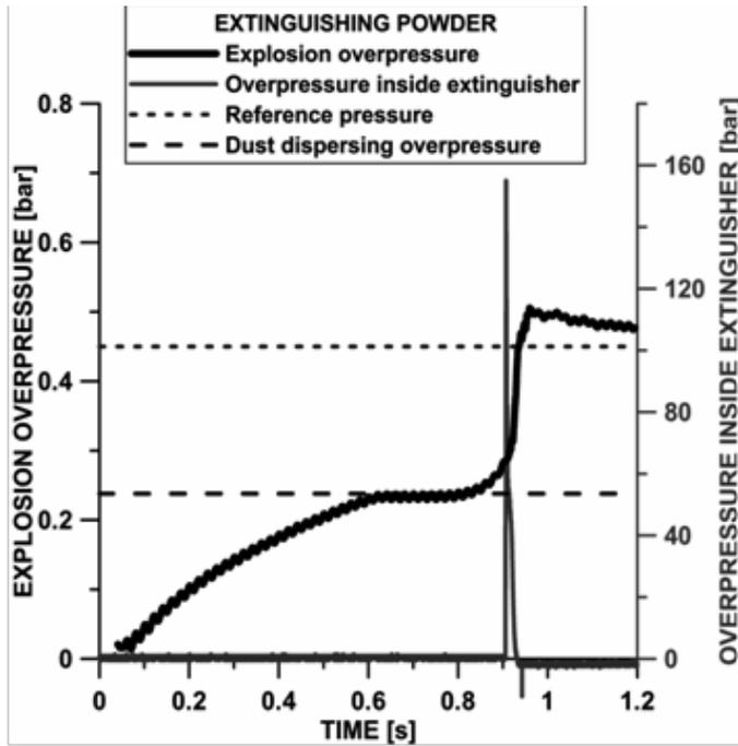
Figure 11: Courses of the overpressure inside the 1.3 m<sup>3</sup> test chamber during explosion of corn starch dust ( $C = 0.2 \text{ kg/m}^3$ ) and inside the extinguisher. Activation from photodiode signal at the level of 0.6 V. Explosion overpressure  $\Delta P = 0.055 \text{ bar}$
