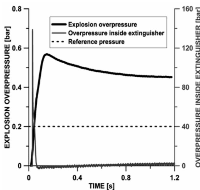
Figure 18: Courses of the overpressure inside the 1.3 m<sup>3</sup> test chamber during explosion of a methane-air mixture (8.5% CH<sub>4</sub>). Activation from photodiode signal at the level of 0.3 V. Explosion overpressure  $\Delta P = 0.37$  bar
