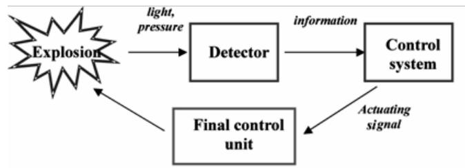
Figure 1: Principle of operation of the suppression system
