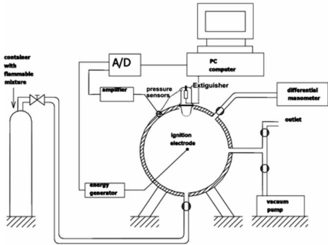
Figure 6: Schematic diagram of the research stand with 1.3 m<sup>3</sup> explosion chamber – for investigation of gaseous explosion suppression
