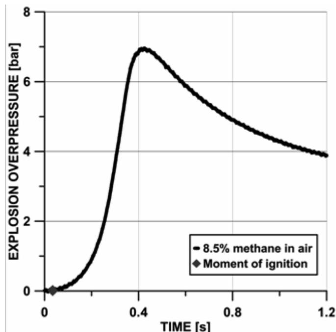
Figure 17: Courses of the overpressure inside the 1.3 m<sup>3</sup> test chamber during explosion of a methane-air mixture (8.5% CH<sub>4</sub>)
