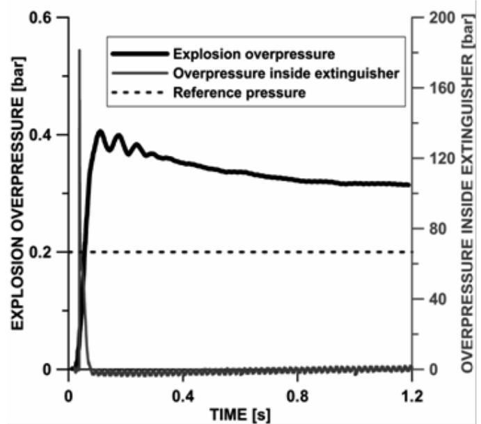
Figure 16: Courses of the overpressure inside the 1.3 m<sup>3</sup> test chamber during explosion of a methane-air mixture (7.5% CH<sub>4</sub>). Activation from photodiode signal at the level of 1.0 V. Explosion overpressure  $\Delta P = 0.21$  bar
