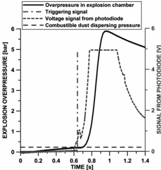
Figure 9: Courses of the overpressure inside test chamber and photodiode voltage signal obtained during explosion of the corn starch dust ( $C = 0.2 \text{ kg/m}^3$ ), without suppression. Explosion overpressure  $\Delta P = 5.7 \text{ bar}$
