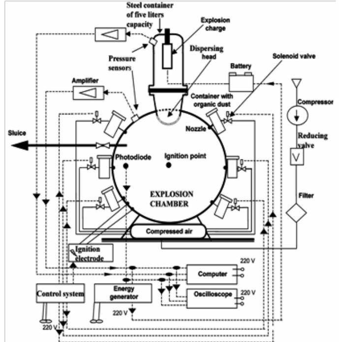
Figure 3: Schematic diagram of the research stand with 1.3 m<sup>3</sup> explosion chamber – for dust explosion investigations
