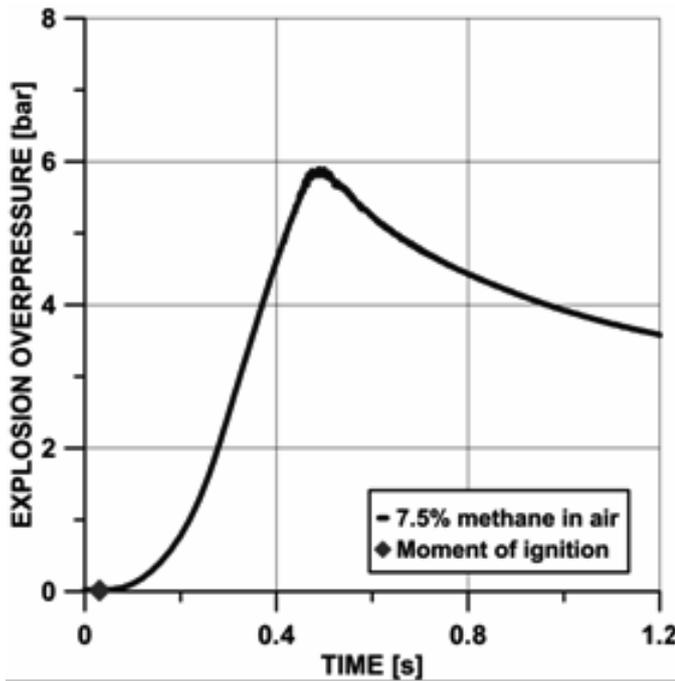
Figure 13: Courses of the overpressure inside the 1.3 m<sup>3</sup> test chamber during explosion of a methane-air mixture (7.5% CH<sub>4</sub>)
