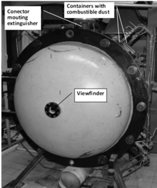
Figure 2: Explosion chamber with 1.3 m<sup>3</sup> volume
