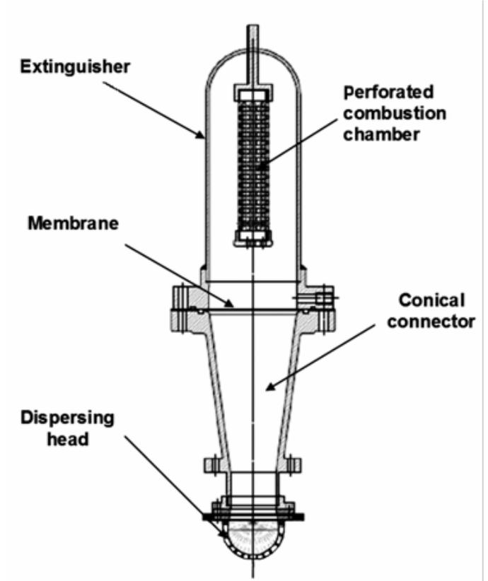
Figure 7: Schematic diagram of the extinguisher
