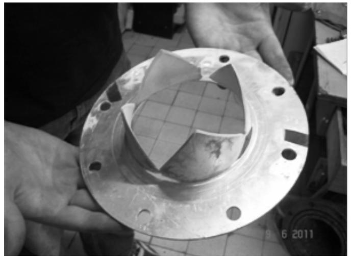
Figure 20: The appearance of the correctly opened membrane after the test
