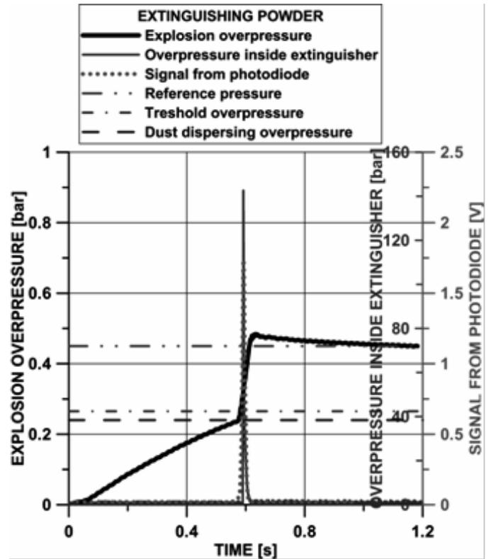
Figure 10: Courses of the overpressure inside the  $1.3 \text{ m}^3$  test chamber during explosion of corn starch dust ( $C = 0.2 \text{ kg/m}^3$ ) and inside the extinguisher. Activation from photodiode signal at the level of 0.3 V. Explosion overpressure  $\Delta P = 0.035 \text{ bar}$
