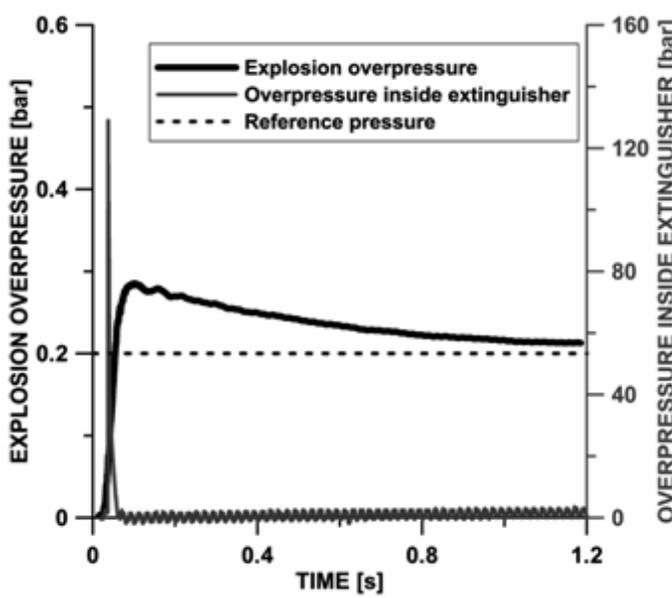
Figure 15: Courses of the overpressure inside the 1.3 m<sup>3</sup> test chamber during explosion of a methane-air mixture (7.5% CH<sub>4</sub>). Activation from photodiode signal at the level of 0.6 V. Explosion overpressure  $\Delta P = 0.075$  bar
