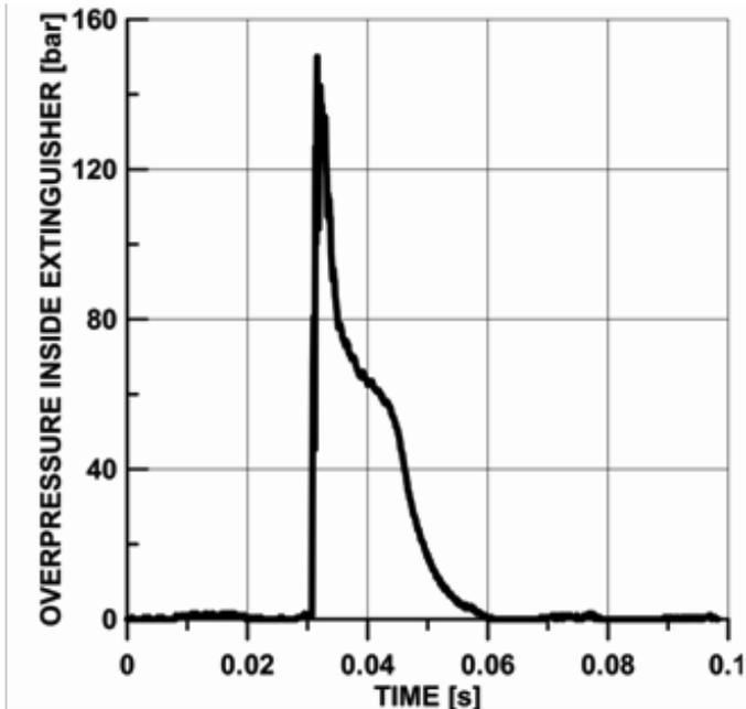
Figure 19: Example course in fire extinguisher pressure recorded during the test explosion suppression
