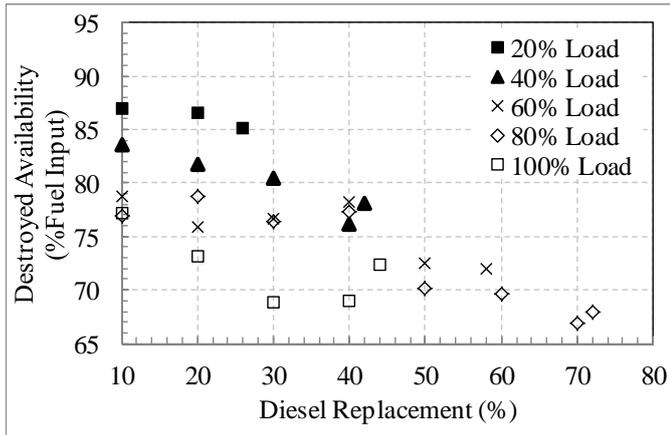
Figure 14: Variation of destroyed availability with diesel replacement
