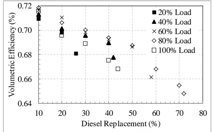
Figure 5: Variation of volumetric efficiency with diesel replacement
