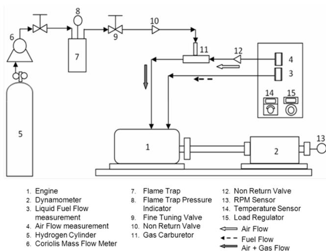
Figure 1: Schematic diagram of the setup
