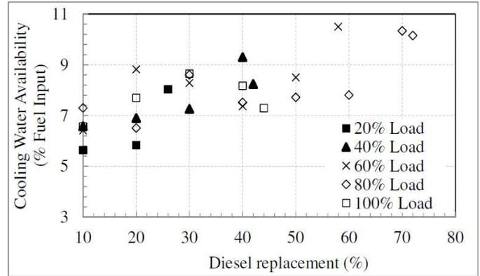
Figure 12: Variation of cooling water availability with diesel replacement
