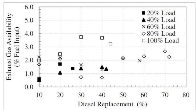
Figure 13: Variation of exhaust gas availability with diesel replacement
