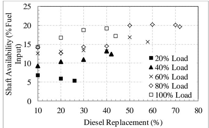
Figure 10: Variation of shaft availability with diesel replacement
