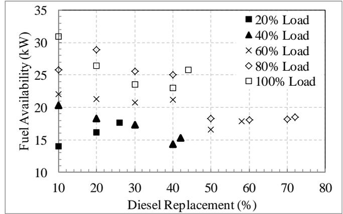
Figure 9: Variation of fuel availability with diesel replacement
