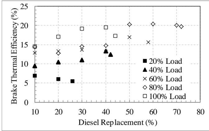
Figure 3: Variation of brake thermal efficiency with diesel replacement
