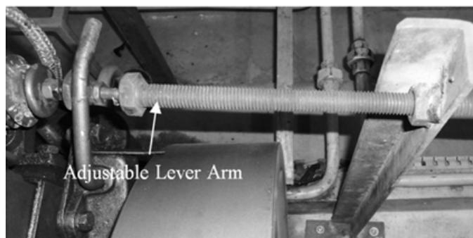
Figure 2: Adjustable lever arm arrangement
