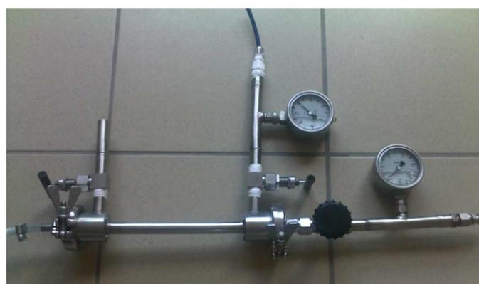
Figure 6: The view of the membranous module with the ceramic-membrane with the measuring instrumentation
