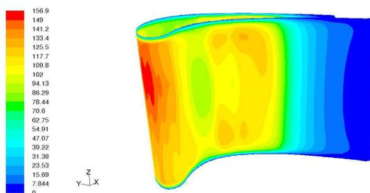
Figure 10: Distribution of Surface Transfer Coefficient – concave side
