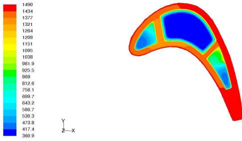
Figure 6: Distribution of a temperature inside the blade
