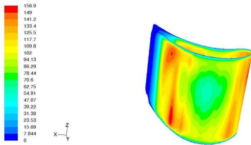
Figure 9: Distribution of Surface Transfer Coefficient—convex side
