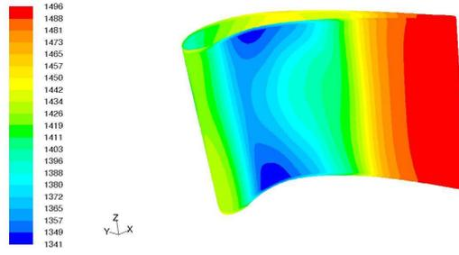
Figure 7: Distribution of temperature on the concave face of the blade
