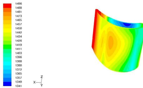
Figure 8: Distribution of temperature on the convex face of the blade
