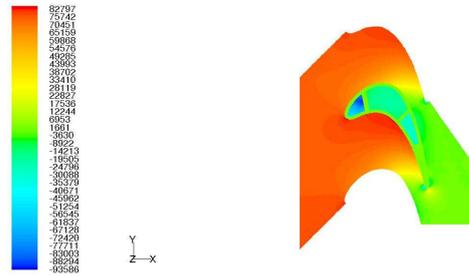
Figure 4: Distribution of static pressure inside and around the blade
