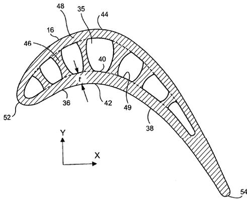
Figure 1: Geometry of the turbine blade
