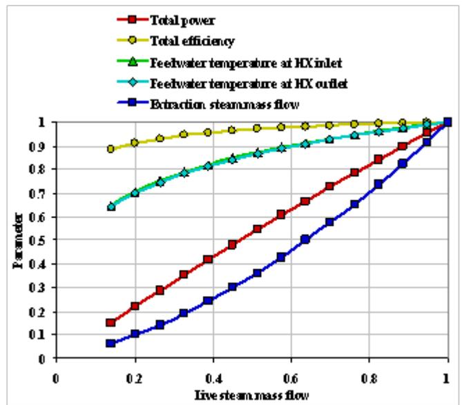
Figure 8: Steam turbine characteristics during off-design operation
