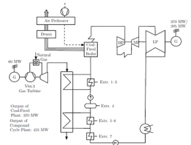
Figure 4: Example of use of a gas turbine to regenerate the coal boiler feedwater [4]
