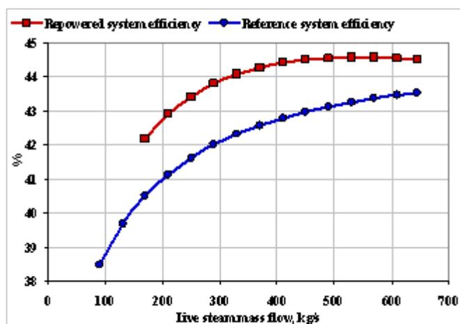
Figure 12: Comparison between steam cycle efficiency and repowered steam cycle efficiency
