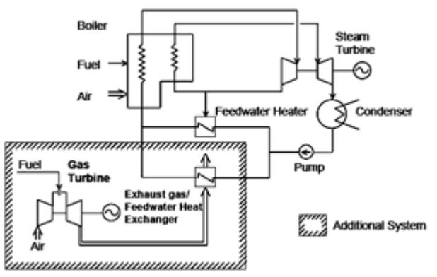
Figure 1: Schematic diagram of using a gas turbine to repower a coal fired power plant to cover peak loads [1–3]
