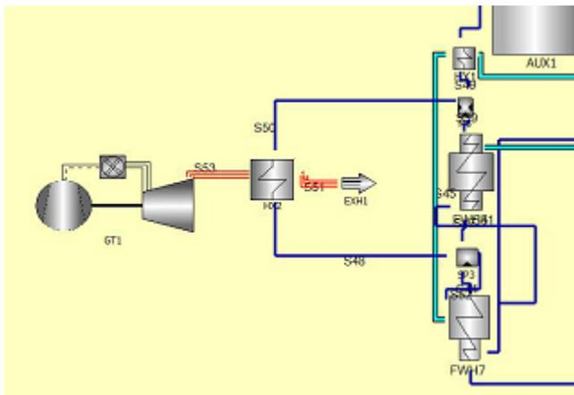
Figure 9: Connection of the gas turbine with the steam system
