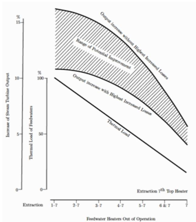
Figure 3: Effect of replacing selected regenerative heat exchangers to increase the power of a steam turbine [4]
