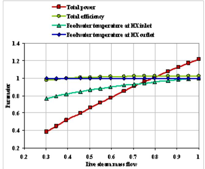
Figure 10: Characteristics of the steam cycle with feedwater repowering
