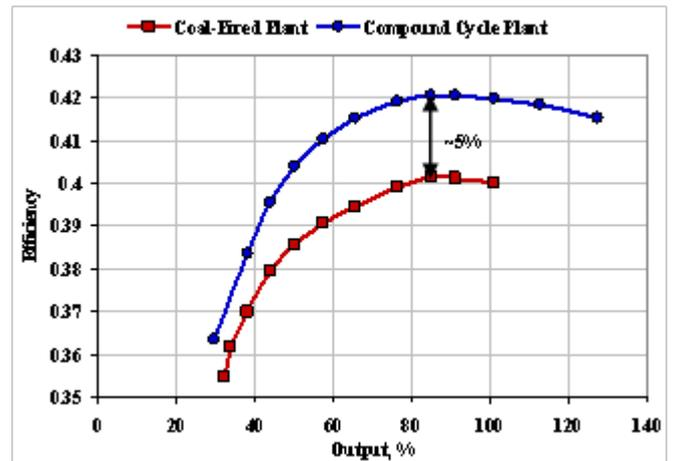
Figure 2: Use of feedwater repowering to increase the efficiency of the steam turbine cycle
