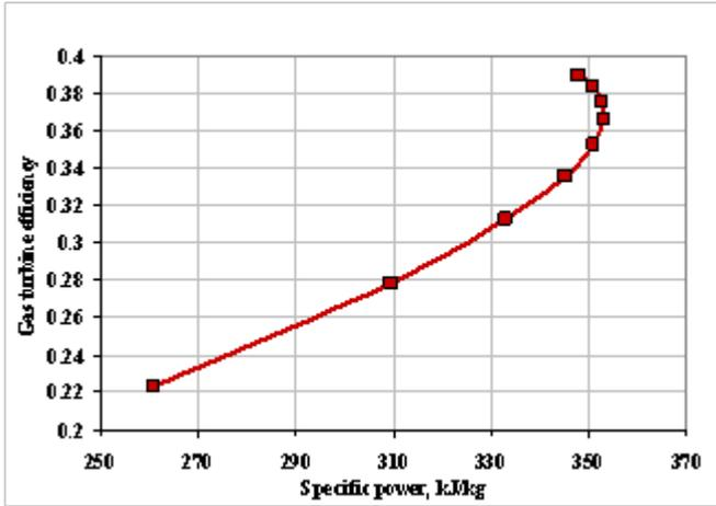
Figure 6: The characteristics of the gas turbine in simple cycle - thermal efficiency and specific power
