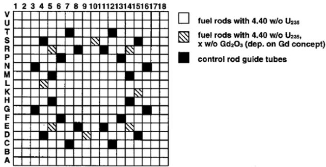
Figure 1: 18x18 U/Gd-fuel assembly with 8 Gd fuel rods [2]
