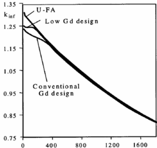
Figure 2: Reactivity characteristics of uranium (U), conventional U/Gd and optimized U/Gd fuel assemblies [2]
