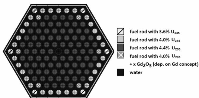
Figure 6: Fuel assembly Gd-2 design, wt. % of GdO depends on Gd concept
