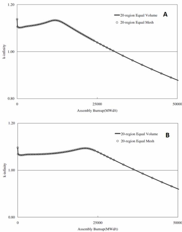
Figure 4: K depending on burnup of PWR fuel assembly 17×17 with burnup (A) 48 GWd/tHM and (B) 55 GWd/tHM
