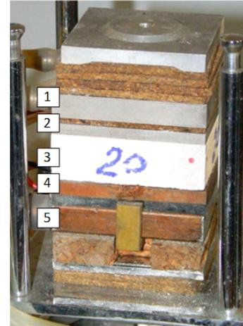
Figure 2: Measurement stack in plate apparatus; 1 – hot plate, 2 – electric heater, 3 – sample, 4 – copper plate, 5 – cold plate
