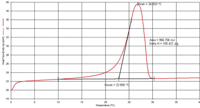
Figure 1: DSC curve for Micronal DS 5008 X
