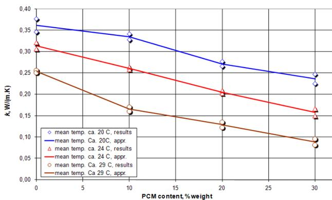
Figure 4: Thermal conductivity of gypsum-PCM composites as a function of PCM concentration
