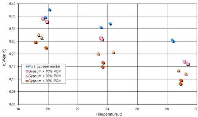
Figure 3: Thermal conductivity of gypsum-PCM composites as a function of temperature
