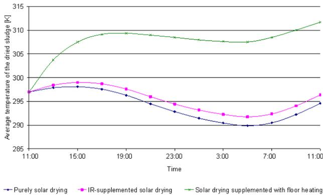
Figure 2: Comparison of average temperature of the dried sludge layer during the modeled days – for purely solar drying, IR-supplemented solar drying and solar drying supplemented with floor heating
