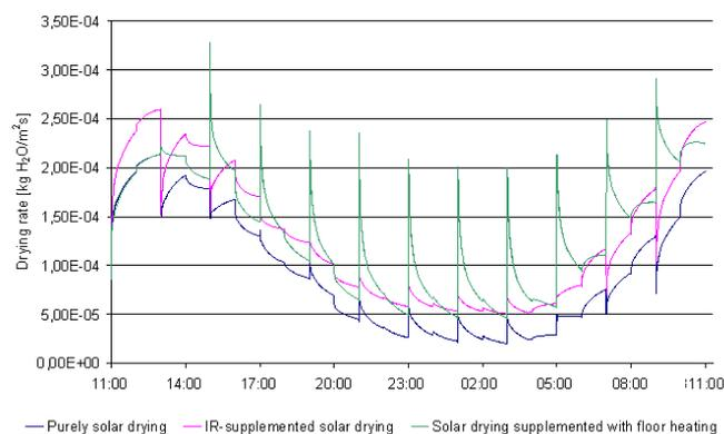
Figure 1: Comparison of drying rate curve for purely solar drying, IR-supplemented solar drying and solar drying supplemented with floor heating
