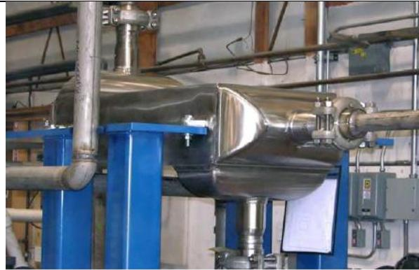
Fig. 14 S-CO<sub>2</sub> high temperature PCHE recuperator at Sandia National Laboratories [63]
