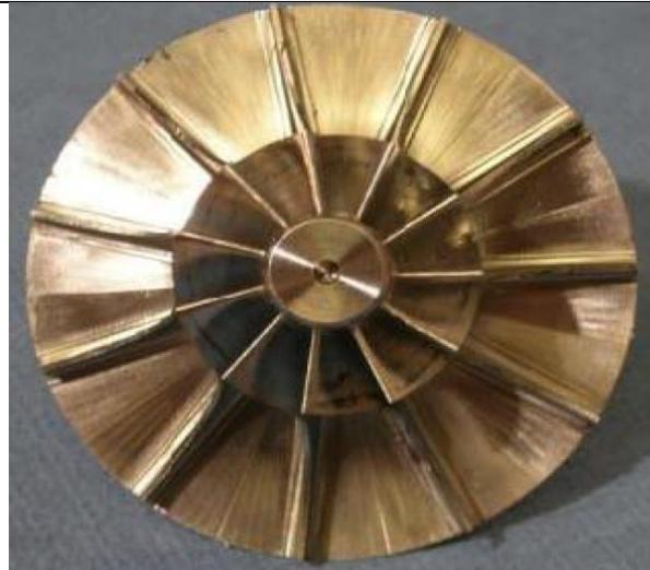
Fig. 11 Wheel of main compressor turbine
