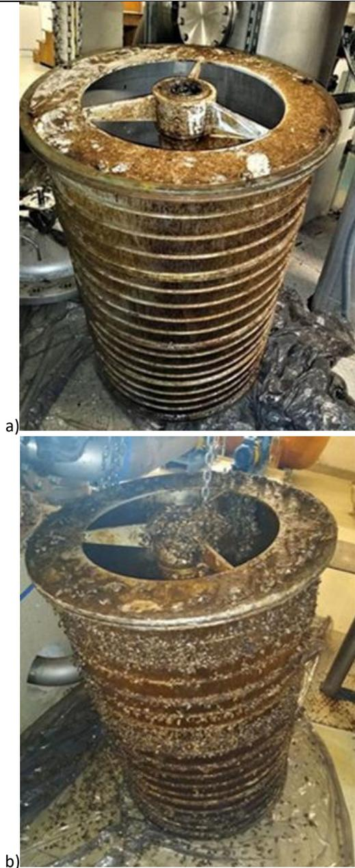
Figure 8: Filter cartridges after operational test: a) cartridge with **nCu** coating, b) standard cartridge without **nCu** coating.
