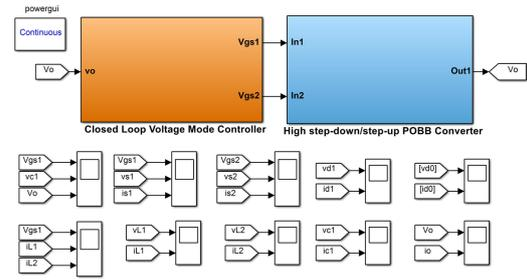
Figure 5: Simulation model of the closed loop voltage mode control POBB converter
