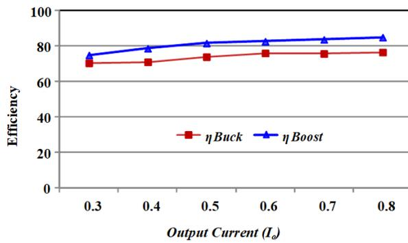
Figure 11: Efficiency vs output current in buck mode and boost mode
