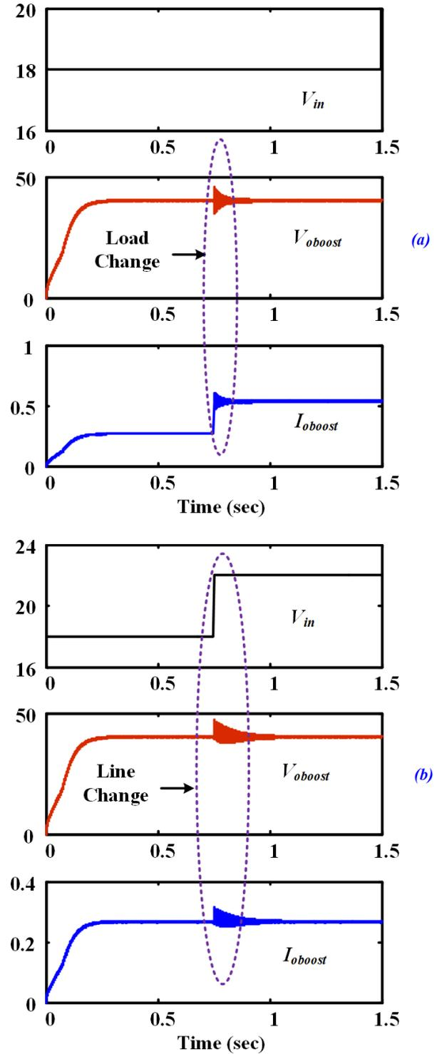
Figure 10: Simulation waveforms of input voltage ( $V_{in}$ ), output voltage ( $V_o$ ) and output current ( $I_o$ ) in boost mode (a) Sudden Change in Load, (b) Sudden change in input voltage.
