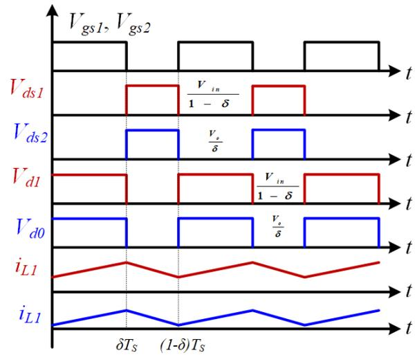
Figure 2: Ideal waveforms of positive output buck-boost converter
