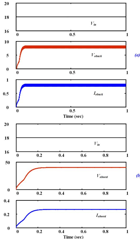
Figure 7: Simulation waveforms of input voltage ( $V_{in}$ ), output voltage ( $V_o$ ) and output current ( $I_o$ ): (a) Buck mode, (b) Boost mode.
