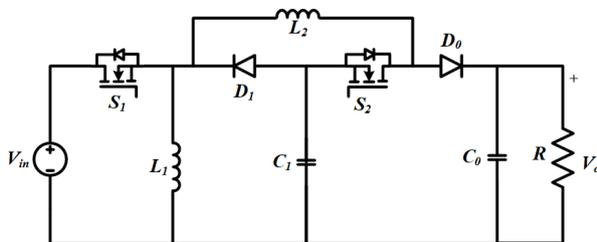
Figure 1: System configuration of positive output buck-boost converter
