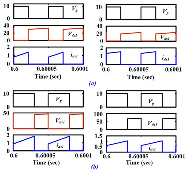
Figure 6: Simulation waveforms of  $V_g$ , switches ( $S_1$  &  $S_2$ ) voltages & currents: (a) Buck mode, (b) Boost mode.
