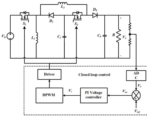
Figure 4: Closed loop voltage mode controlled high gain POBB converter
