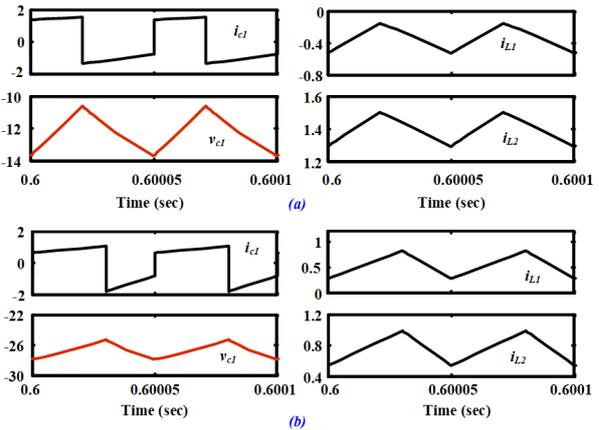
Figure 8: Simulation waveforms of capacitor current ( $i_{C1}$ ), voltage ( $v_{C1}$ ), inductor currents ( $i_{L1}$  &  $i_{L2}$ ): (a) Buck mode, (b) Boost mode.
