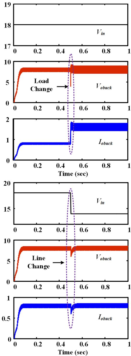
Figure 9: Simulation waveforms of input voltage ( $V_{in}$ ), output voltage ( $V_o$ ) and output current ( $I_o$ ) in buck mode (a) Sudden Change in Load, (b) Sudden change in input voltage.
