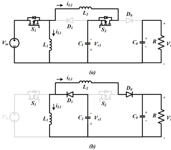
Figure 3: Equivalent circuits of the POBB converter. (a) Mode 1. (b) Mode 2
