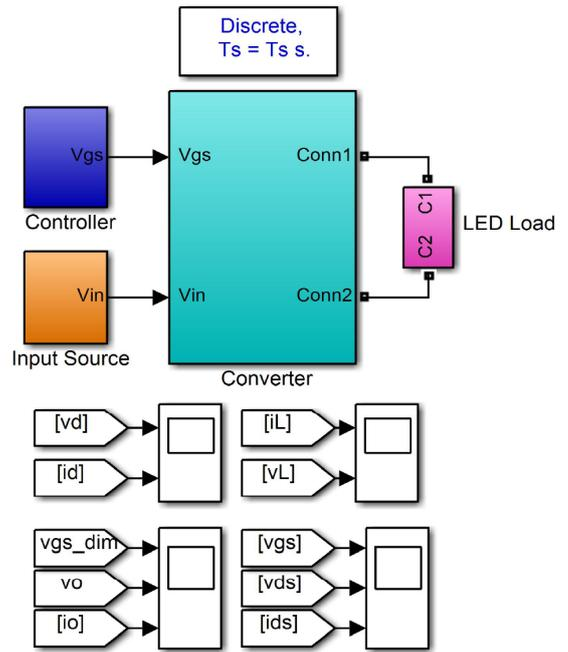
Figure 6: Simulation model of dimmable boost LED driver, open loop model
