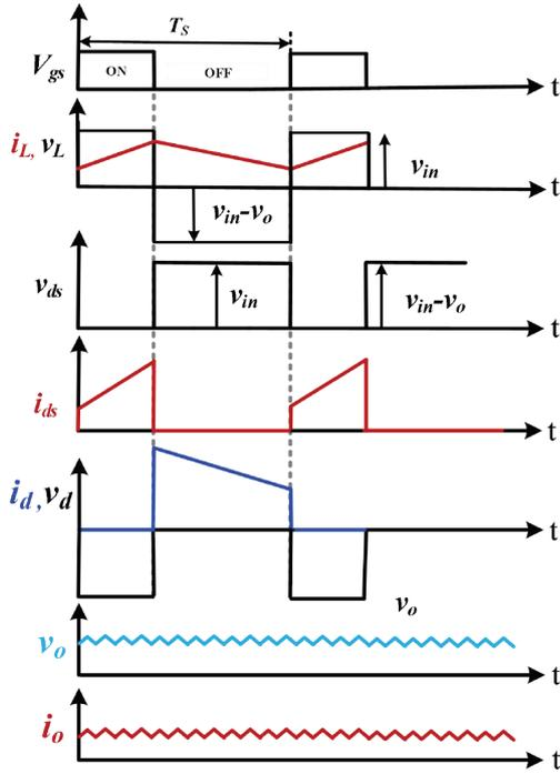
Figure 2: Idealized waveforms of dimmable boost LED driver
