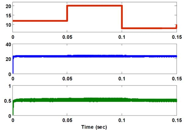
Figure 11: Closed loop waveforms for input variations, input voltage (top trace), output voltage (middle trace) and output current (bottom trace)
