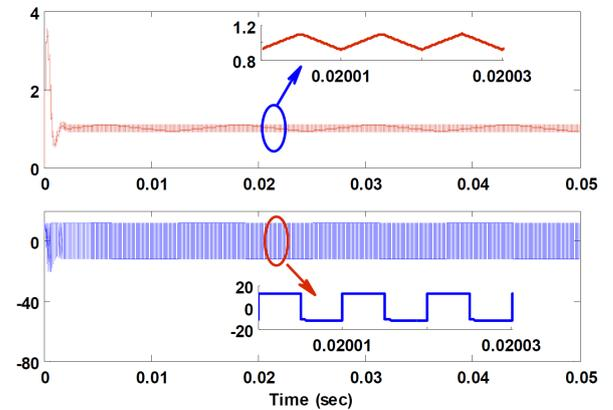
Figure 9: Inductor current (top trace) and inductor voltage (bottom trace)
