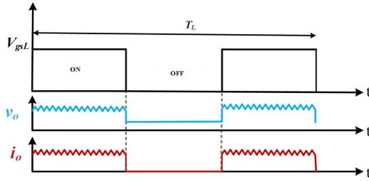
Figure 5: Dimming pulse, output voltage and current of dimmable boost LED driver
