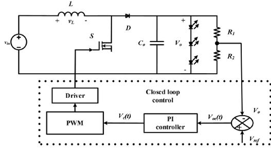
Figure 4: Closed loop voltage mode control boost LED driver
