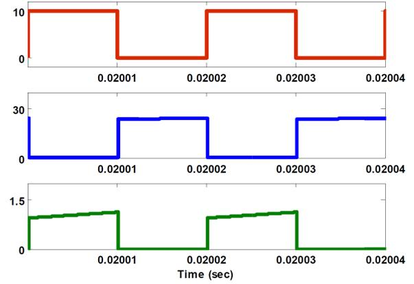
Figure 8: Gate pulse (top trace), switch voltage (middle trace) and switch current (bottom trace)
