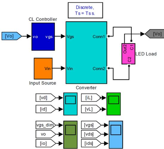
Figure 7: Simulation model of dimmable boost LED driver, closed loop model
