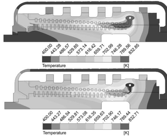
Figure 4: Distribution of the temperature field in the 180th minute of start-up 3h. Top: starting without injection of a cooling steam. Bottom: starting with injection of a cooling steam
