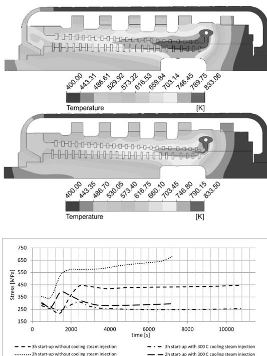
Figure 6: H-M-H stress course during turbine start-up
