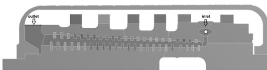
Figure 2: Reference model of the WP part of the 18K390 turbine with marked inlet and outlet edges
