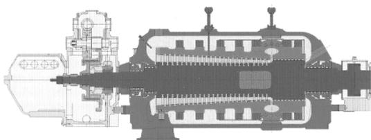
Figure 1: Cross section of the turbine's 18K390 HP part [4]
