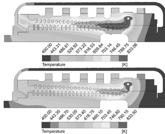
Figure 5: Distribution of the temperature field in the 120th minute of start-up 2h. Top: starting without injection of a cooling steam. Bottom: starting with injection of a cooling steam
