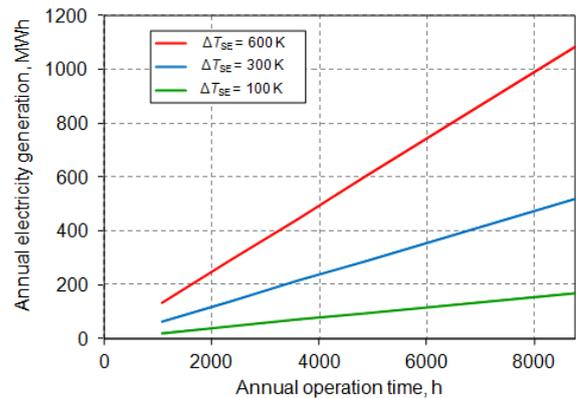
Figure 6: Annual electricity generation as a function of operation time
