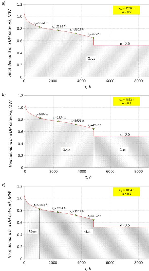
Figure 4: Distribution of heat demand over the network for CHP ( $Q_{CHP}$ ) and additional heat source ( $Q_{AB}$ ) for  $\alpha = 0.5$  and various annual operating time
