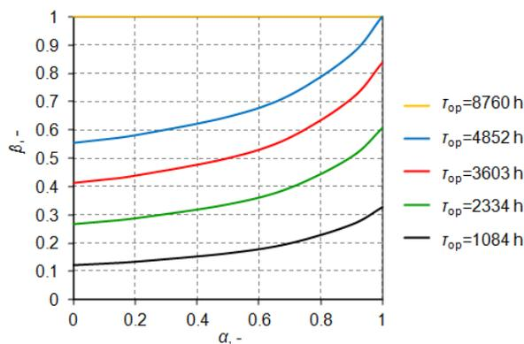
Figure 7: The relationship between  $\beta$  and  $\alpha$  coefficients for various CHP system configurations
