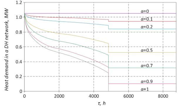
Figure 2: The annual ordered heat demand curve in the analyzed network as a function of coefficient  $\alpha$
