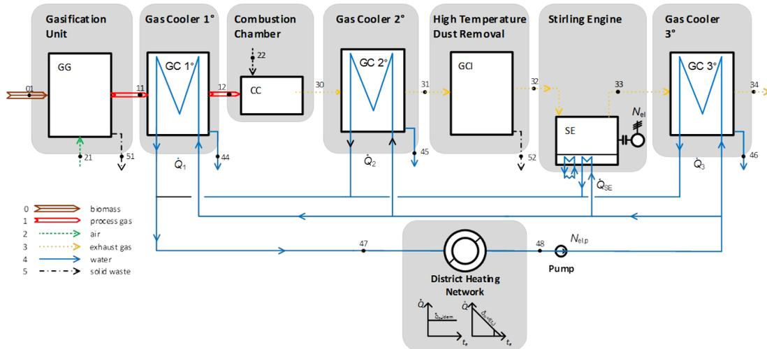
Figure 1: A schematic diagram of a DH system integrated with biomass gasification and Stirling engine; Denotations: GG—gas generator, GC—gas cooler, GCI—gas cleaning unit, SE—Stirling engine
