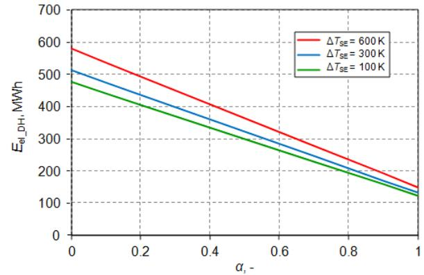
Figure 3: The annual demand for electricity in the analyzed district heating network for various values of  $\Delta T_{SE}$
