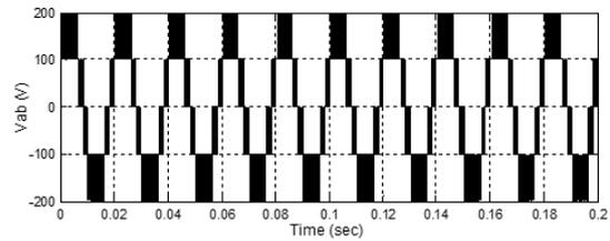
Figure 10: Simulation result of the output line voltage waveform of T-type inverter at modulation index ( $M_i$ ) = 0.907
