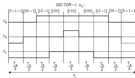
Figure 6: Nine segment switching-diagram
