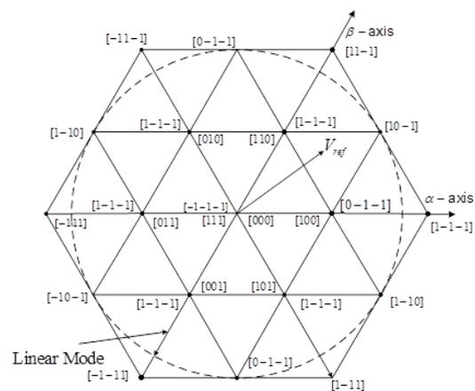
Figure 3: Space vector diagram of a 3-level inverter
