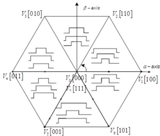
Figure 7: Switching Patterns for Six Sectors inside the Circle with nine segment implementation
