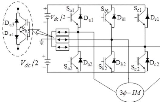
Figure 2: T-type 3-level 3-phase inverter with motor load
