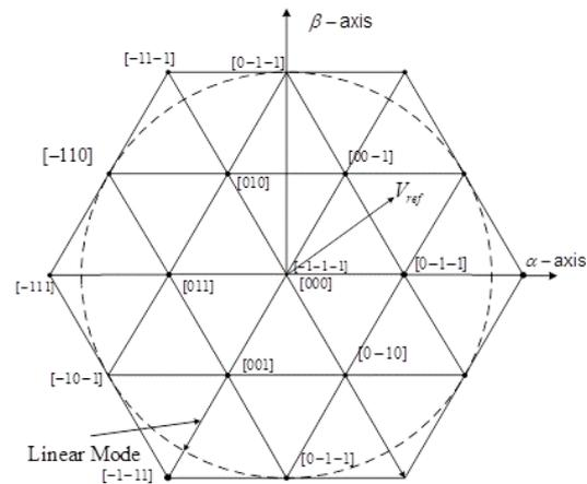
Figure 8: Space diagram condition for faulty phase-A
