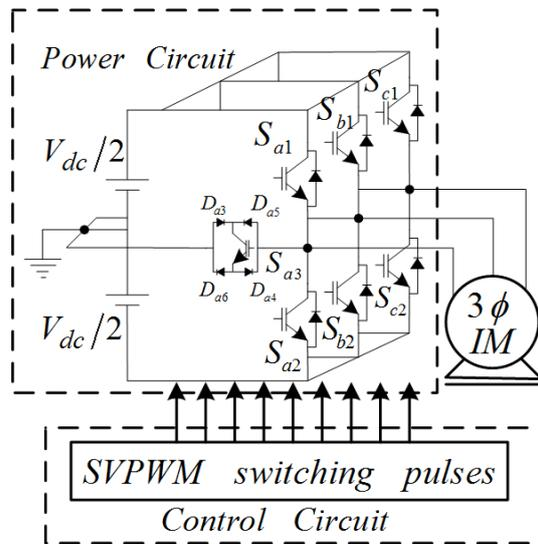
Figure 1: Overall schematic diagram of the proposed topology
