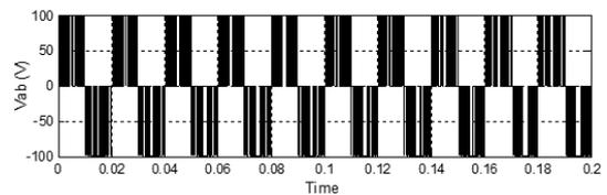
Figure 12: Simulation result of the output voltage waveform of T-type inverter with modulation index ( $M_i$ ) = 0.454
