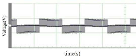
Figure 13: Experimental result of the output voltage waveform ( $V_0 = V_{ab} = 100\text{V} : 100\text{V/div.}$ ) of T-type inverter with modulation index ( $M_i$ ) = 0.454
