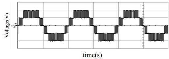
Figure 11: Experimental result of the output voltage waveform ( $V_0 = V_{ab} = 200V : 100V/div.$ ) of T-type inverter with modulation index ( $M_i$ ) = 0.907
