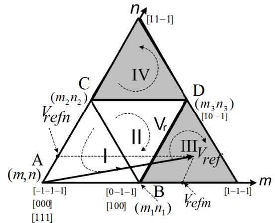
Figure 5: Switching sequence pattern of the voltage vector
