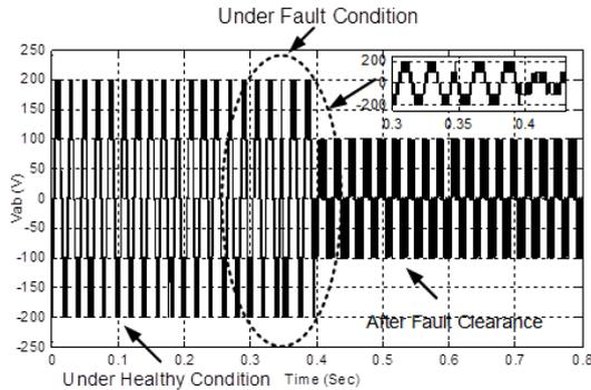
Figure 9: Modes of operation i.e. under normal operation mode, faulty operation mode, fault tolerant operation mode
