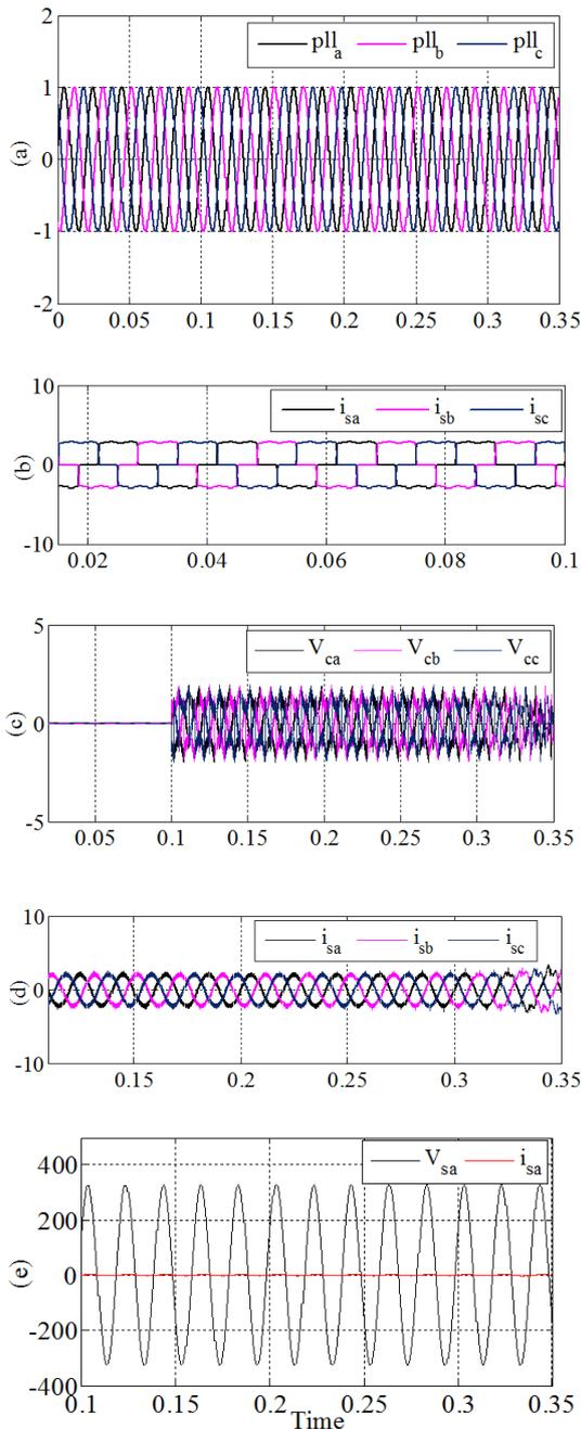
Figure 5: Simulation results for SAPF under nonlinear load condition (a) load current before compensation (b) PLL synchronization output current (c) source current after SAPF (d) compensation current by SAPF (e) phase relation between source voltage and source current.
