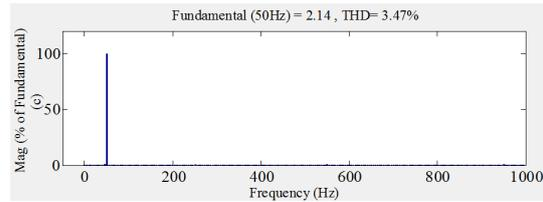
Figure 11: Frequency spectrum of source currents (phase a, phase b phase c respectively) after compensation for RD-FLC based APF with non linear
