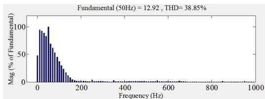
Figure 10: Frequency spectrum of source current before compensation for three phase SAPF with non linear load
