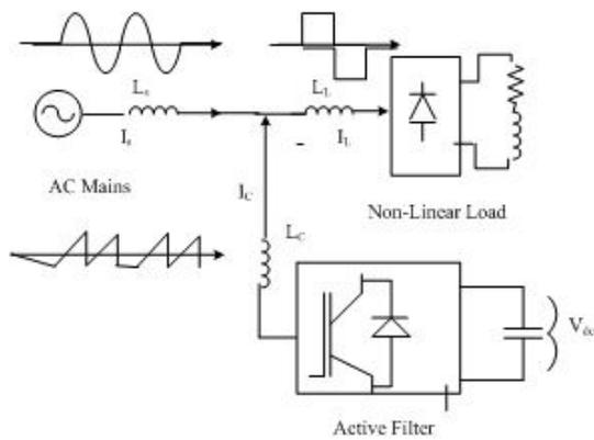
Figure 1: Basic shunt active power filter
