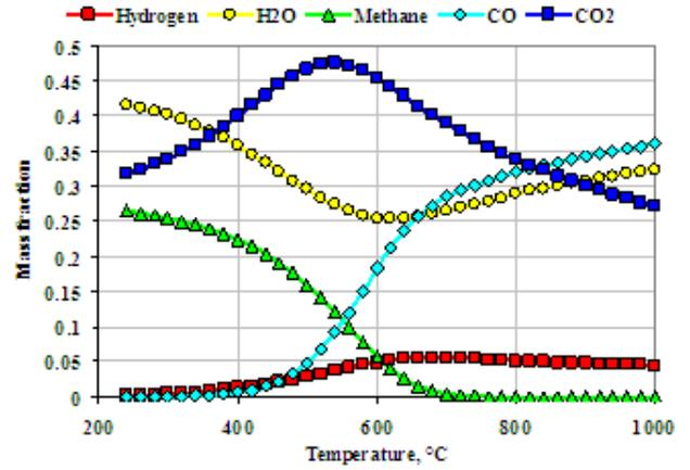
Figure 2: Canola Oil Syngas composition as a function of temperature
