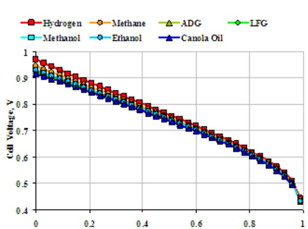
Figure 7: MCFC cell voltage vs. fuel utilization factor for various biofuels
