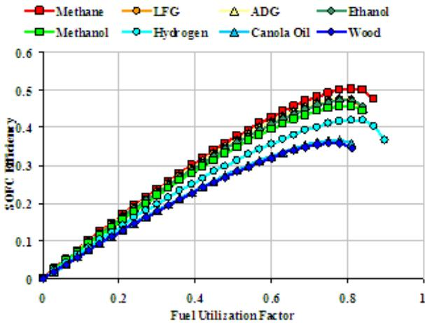
Figure 4: SOFC efficiency vs. fuel utilization factor for various biofuels
