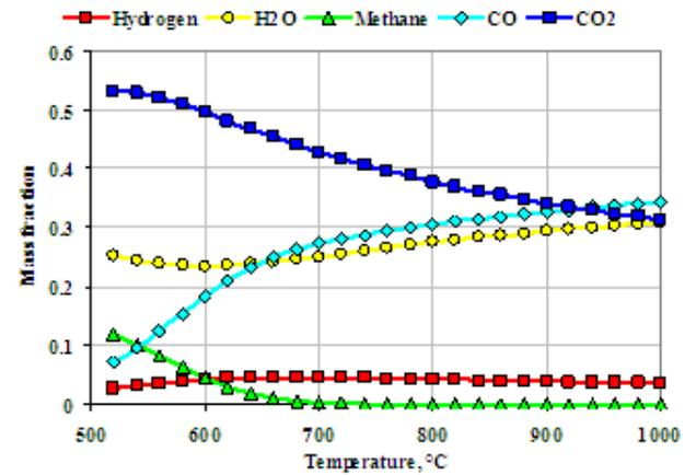
Figure 3: Wood Syngas composition as a function of temperature
