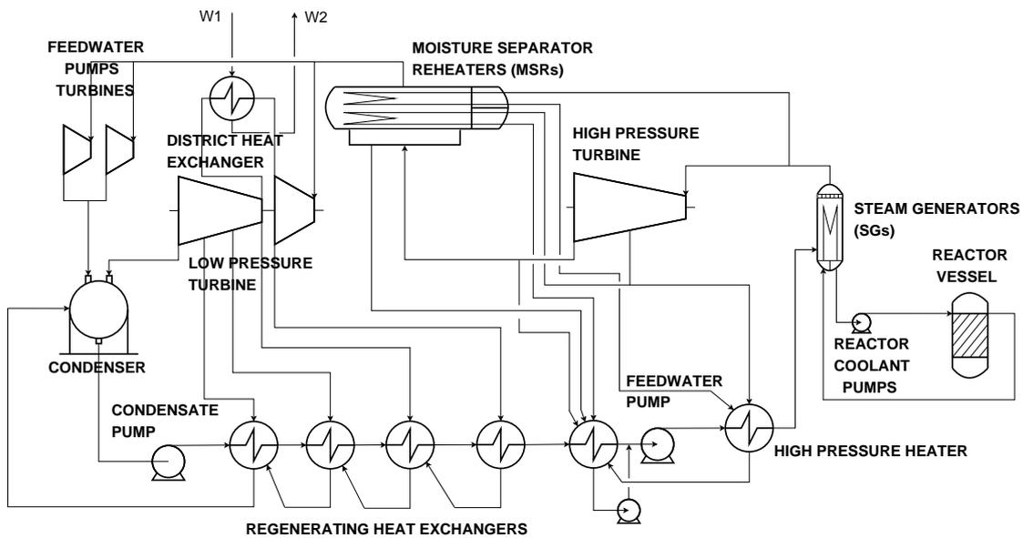
Figure 7: Diagram of NCHP using heat from the bypassed turbine
