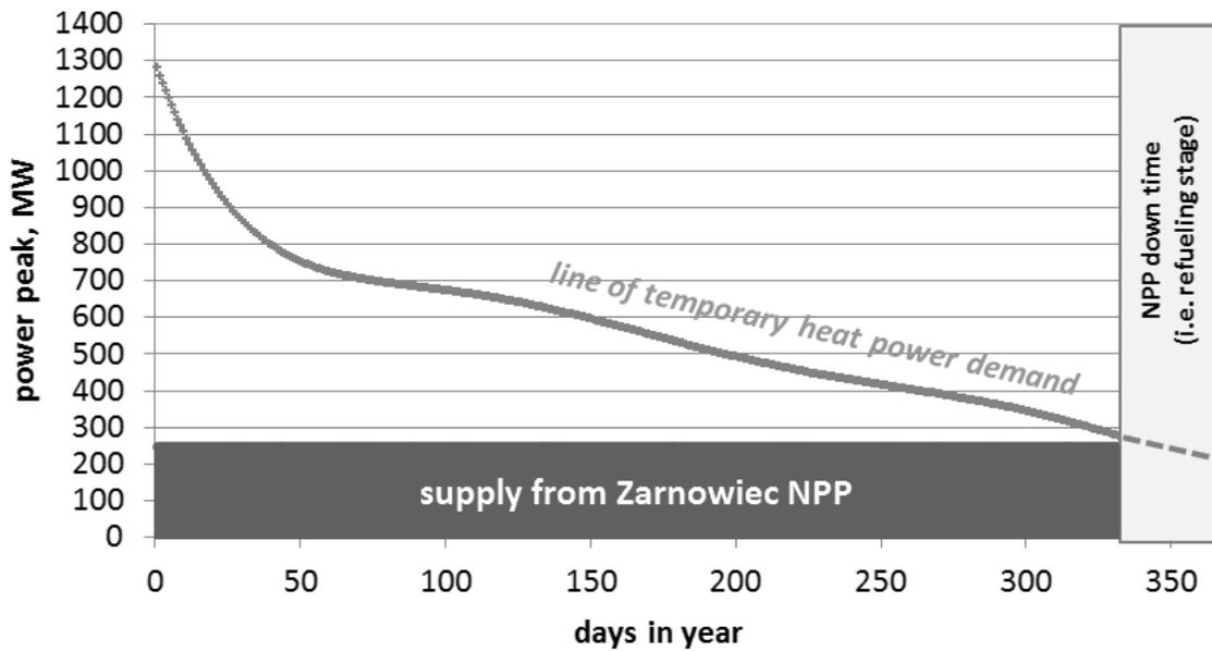
Figure 2: Heat demand and proposed power load of heat network
