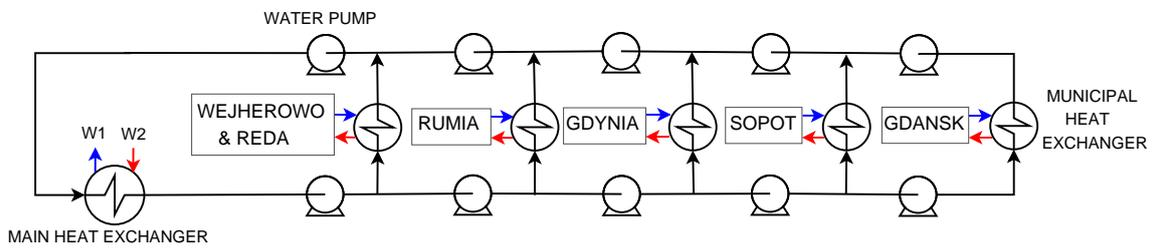
Figure 5: Diagram of the district heating network
