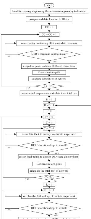
assign load points to chosen DERs and cluster them Construct micro-grids V calculate the total cost of network V  $R < N_R$ ves ¥ no Calculate total cost of I-th imperialist ¥  $I \le N_1$ yes ¥ no change the positions of imperialist and colony which it's cost is lower eliminate weak empire and give its colony to powerful empire ۲ eliminate the empire with no colony Ý (D<number of decades) end no
