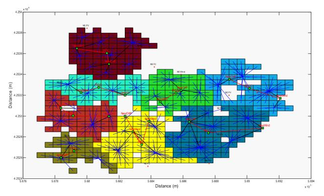
Figure 5: Clustering greenfield distribution network into multiple autonomous MGs (8 MG with specific electrical boundary)
