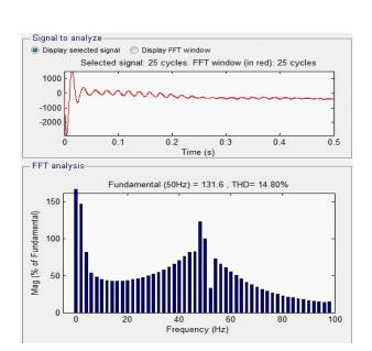
Figure 26: Harmonic spectrum of isq current SVPWM
