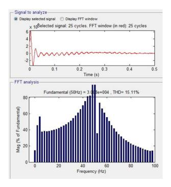
Figure 28: Harmonic spectrum of active power SVPWM
