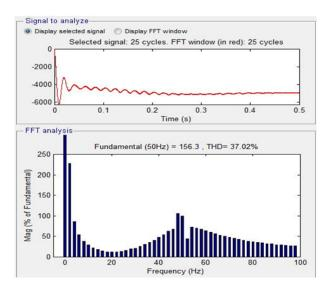
Figure 23: Harmonic spectrum of isd current SPWM
