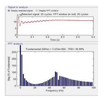
Figure 29: Harmonic spectrum of reactive power SPWM
