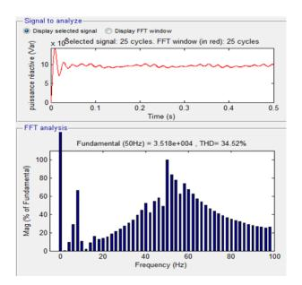
Figure 30: Harmonic spectrum of reactive power SVPWM
