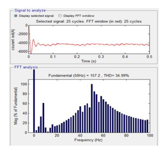
Figure 24: Harmonic spectrum of isd current SVPWM
