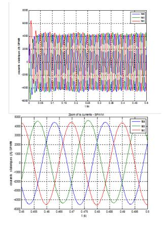
Figure 13: Stator currents is—SPWM
