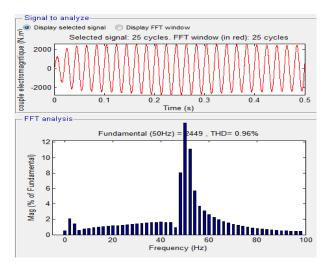
Figure 22: Harmonic spectrum of electromagnetic torque SVPWM
