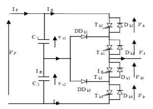
Figure 2: Modeling structure of one inverter arm
