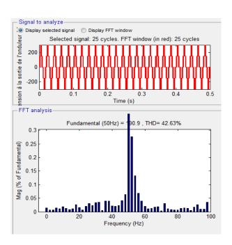
Figure 20: Harmonic spectrum of output inverter Voltage SVPWM
