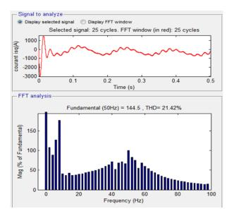
Figure 25: Harmonic spectrum of isq current SPWM
