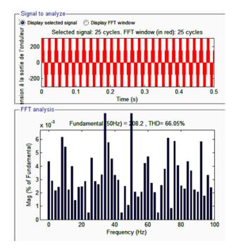
Figure 19: Harmonic spectrum of output inverter Voltage SPWM
