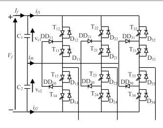
Figure 1: Three level inverter structure
