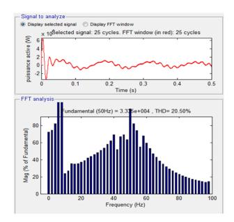
Figure 27: Harmonic spectrum of active power SPWM
