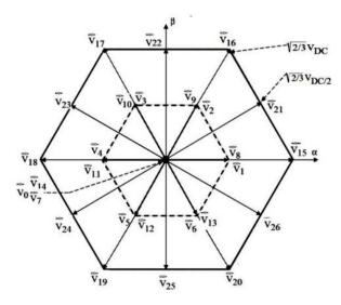
Figure 4: Three level inverter hexagons [13]
