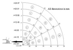
Figure 2: Slice of core conductor delimited by two  $90^\circ$  inclined planes divided into arc formed components
