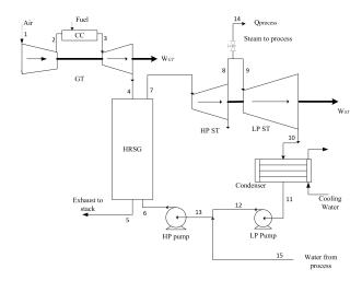
Figure 1: Layout of extraction steam turbine cycle
