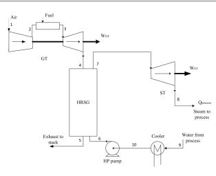
Figure 2: Layout of backpressure steam turbine cycle
