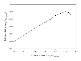
Figure 3: ST efficiency correction characteristic
