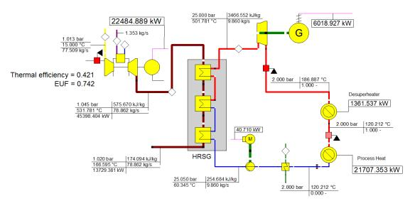
Figure 5: Layout of backpressure steam turbine cycle
