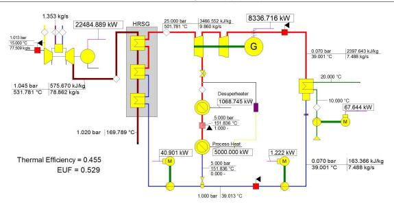
Figure 4: Layout of extraction steam turbine cycle
