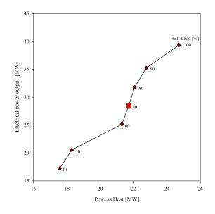
Backpressure Steam Turbine 2 [bar], T<sub>s</sub>= 120 [°C]
