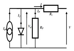
Figure 2: The Equivalent electrical circuit of a photovoltaic cell
