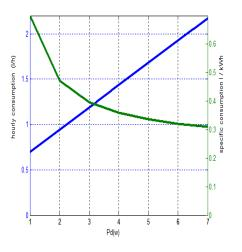
Figure 10: Consumption of the diesel generator as a function of the power produced  $% \left( {{{\bf{F}}_{{\rm{s}}}}} \right)$
