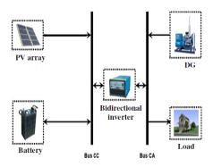
Figure 1: The analyzed hybrid system with a diesel generator DG
