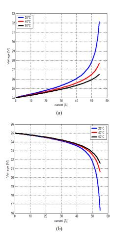
Figure 8: Variation of the voltage versus the current for different values of temperature: a) discharge mode; b) charging mode
