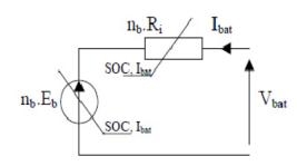
Figure 3: Equivalent electrical diagram of n<sub>b</sub> battery elements in series
