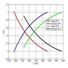
Figure 7: Variation of the SOC versus the capacity for different values of temperature
