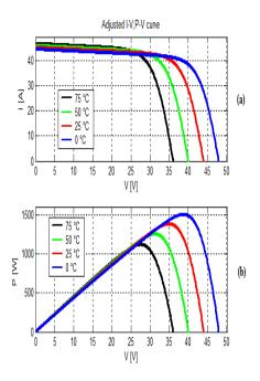
Figure 5: I-V and P-V curves of a PV generator at variable temperature and constant irradiation
