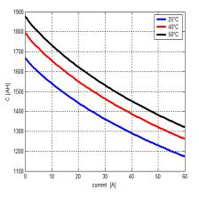
Figure 6: Variation of the capacity versus the current for different values of the temperature
