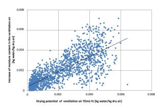
Figure 1: Increase in moisture content in the ventilation air as a function of drying potential for that air during the analyzed operating cycle of the test facility—experimental data
