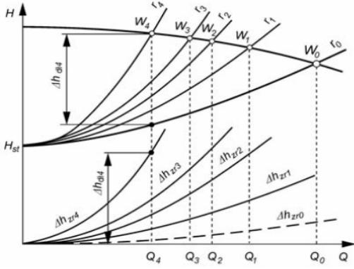
Figure 1: Change in pipeline characteristics  $r = H_p(Q)$  and operating point W of the pump as a result of the change in the control valve opening level [1]
