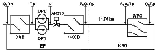
Figure 3: Flow chart of the district heating water closed loop with the measurement point indicated
