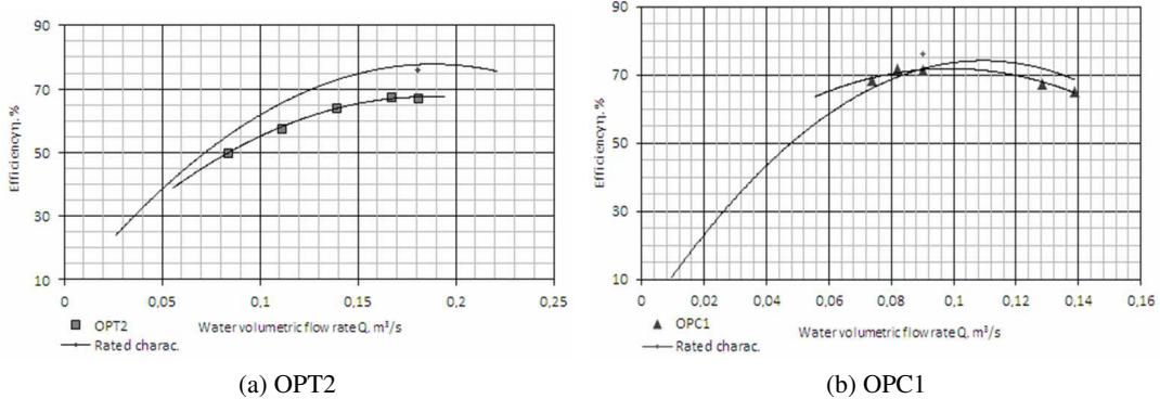
Figure 6: Hot water pump efficiency
