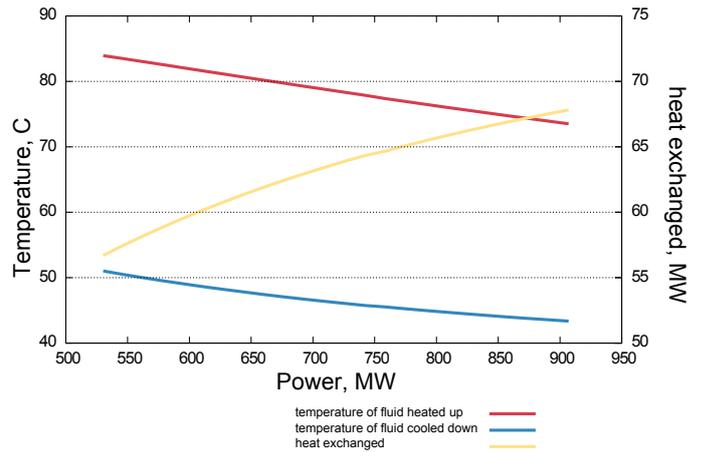
Figure 7: Outlet temperatures of streams which flow through heat exchanger LP1 as a function of power generated
