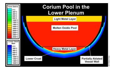
Figure 5: Model of the corium molten pool formation in the lower head of the RPV [7]
