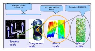
Figure 4: thermal-hydraulic codes for various analysis scale
