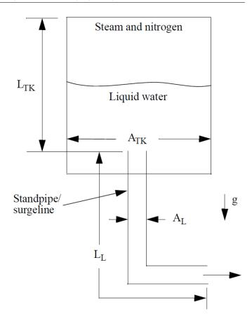
Figure 9: Schematic of a cylindrical accumulator with main components indicated
