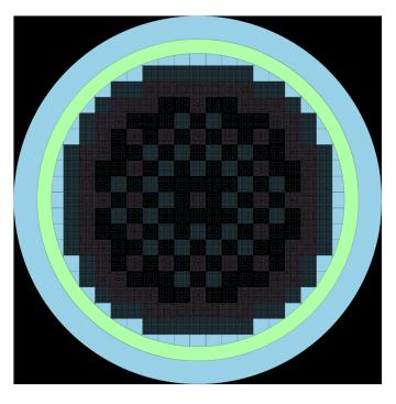
Figure 1: Core cross section analyzed using the Serpent code
