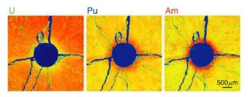
Figure 3: Elements distribution in the 24 hours irradiated %5Am-MOX fuel [3]
