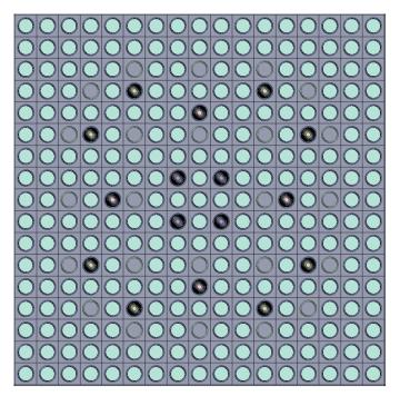
Figure 2: Fuel assembly cross section analyzed in the Serpent code
