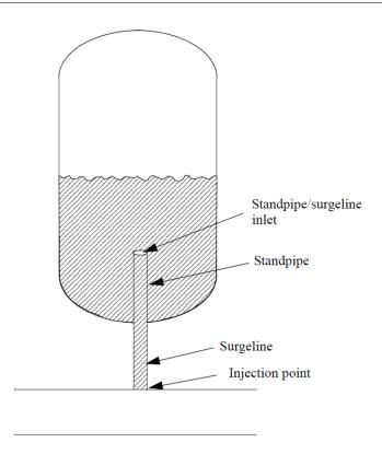
Figure 10: Schematic of an accumulator showing standpipe/surgeline inlet
