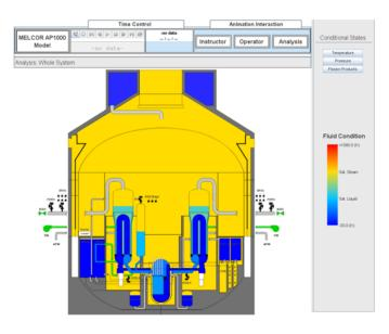
Figure 6: Simulator in the graphic interface connected to the MELCOR code [8]
