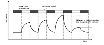
Figure 3: Curve illustrating the measuring signal with keying
