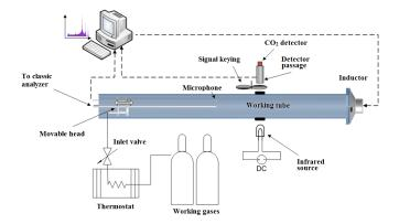
Figure 2: Diagram of the test stand for the analysis of carbon dioxide separation
