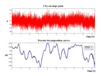
Figure 9: Complete configuration curve after decomposition using db4 and db8 wavelets
