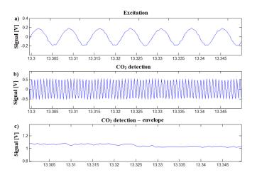
Figure 5: Example of a fragment of the curve in a short time window: a) measuring microphone path, b)  $CO_2$  detection path, c) calculated tube—difference between maximum and minimum values for each cycle
