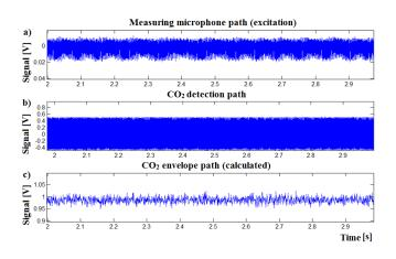
Figure 4: Curves illustrating the real measuring signal: a) measuring microphone path, b)  $CO_2$  detection path c) calculated tube
