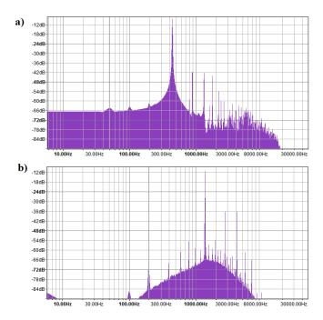
Figure 7: FFT analysis of the complete configuration curve: a) measuring microphone path, b)  $CO_2$  detector path
