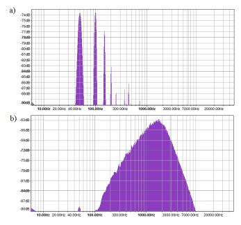
Figure 6: FFT analysis of curves plotted for the incomplete configuration: a) curve recorded by the measuring microphone, b) curve recorded for the  $CO_2$  detection system
